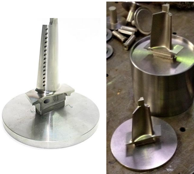
Fig. 5. The cooled blade brazed into the technological plate (on the left) and assembling of capsules
