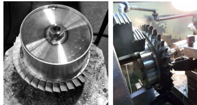
Fig. 3. The capsule with the blisk blank after HIP process (on the left) and the machining of the blisk blank
