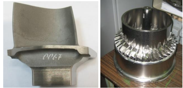
Fig. 2. The single crystal blade (on the left) and the technological ring with blades installed in the equipment for brazing
