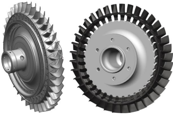
Fig. 1. The prototype wheel (on the left) and the model of the bimetallic blisk
