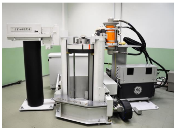
Fig.2. A general view the X-ray tomograph computing VT-600XA.
