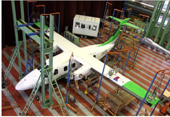
Fig.5. Arrangement of EV-55M aircraft GVT at VZLU
