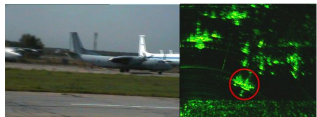
Fig. 2. Monitoring of aircraft AN-24 orientation on taxiway
