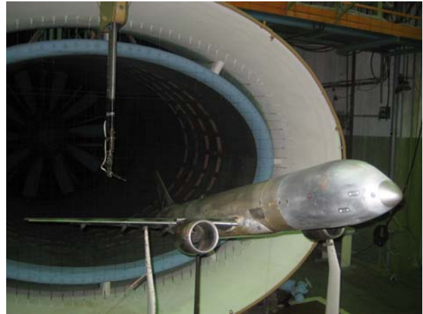
Fig. 2 . The research model in WT T-103 TsAGI
