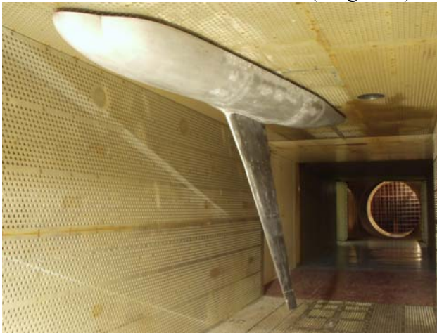
Fig. 1 . The research half model in WT T-128 TsAGI
