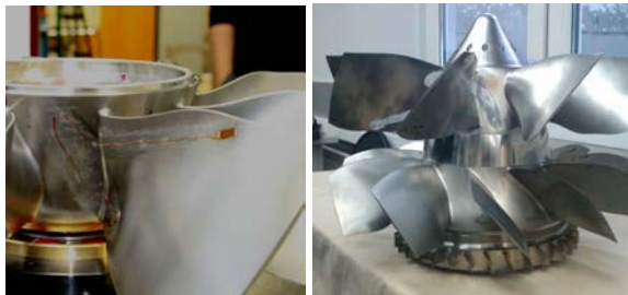
Figure 2: Rotor 1 blisk with strain gauge instrumentation (left) and CRTF2b fan stage assembly (right)
