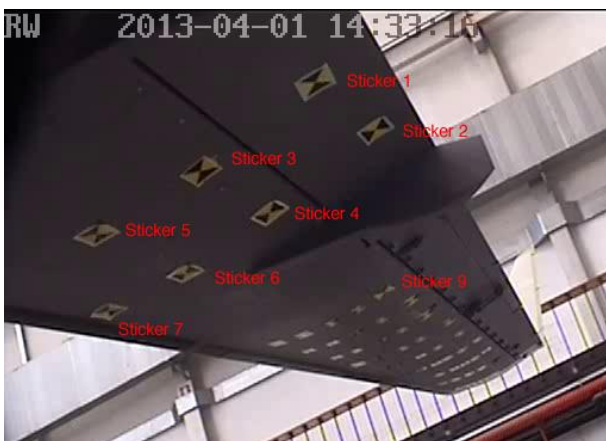
Fig.7: Determination of camera alignment
