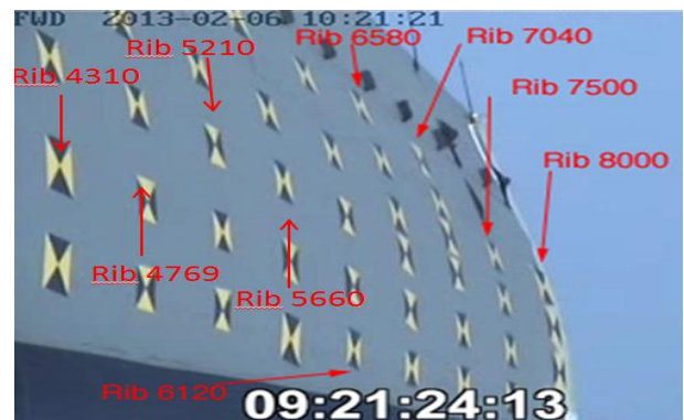
Fig.8: Sticker array on the outer wing's lower surface
