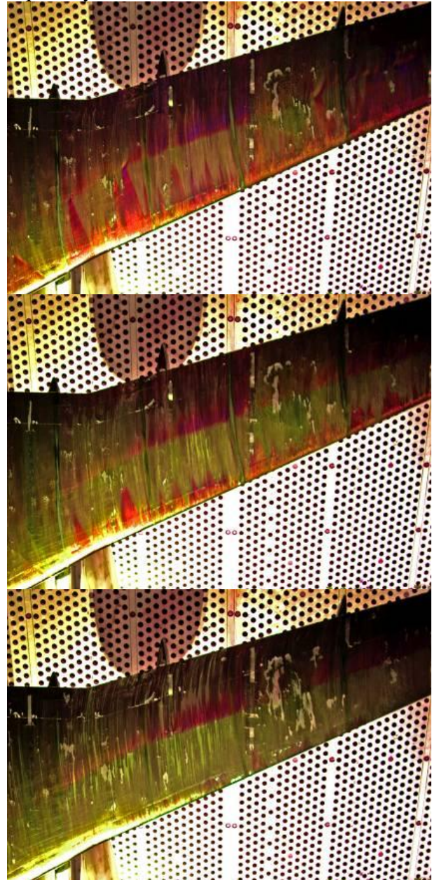
Fig. 5 LC Visualization of Surface Flow at the Metal Wing by Shear Stress Sensitive Liquid Crystals in T-128 Transonic Wind Tunnel (TsAGI), M=0,78 , \alpha = 4,5^\circ , Re = 3 \times 10^6 , 6 \times 10^6 and 9 \times 10^6 Correspondingly
