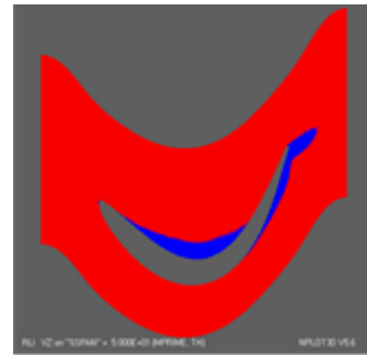
Figure 9: Contours of axial velocity ( V_x ) for HL-A configuration. V_x > 0 is shown in RED. V_x < 0 is shown in BLUE, implying separated flow. ( Re = 140000 , SST with Durbin limiter).
