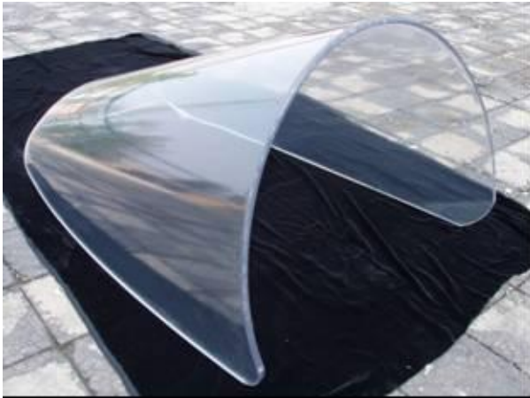
Fig. 7. Polycarbonate aircraft windshield coated with MTMS/TEOS/MEMO coating
