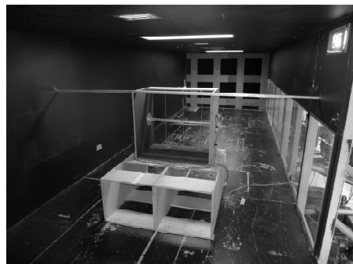
Figure 3 – Pressure tapped airfoil between end plates and upstream of grids in RMIT IWT
