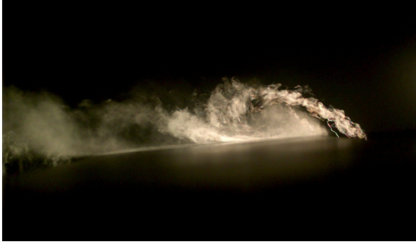
Figure 9: Leading edge separation and enhanced shear layer roll up, leading to the formation of a vortex. AoA = 10Deg, Ti=12.3. [18]
