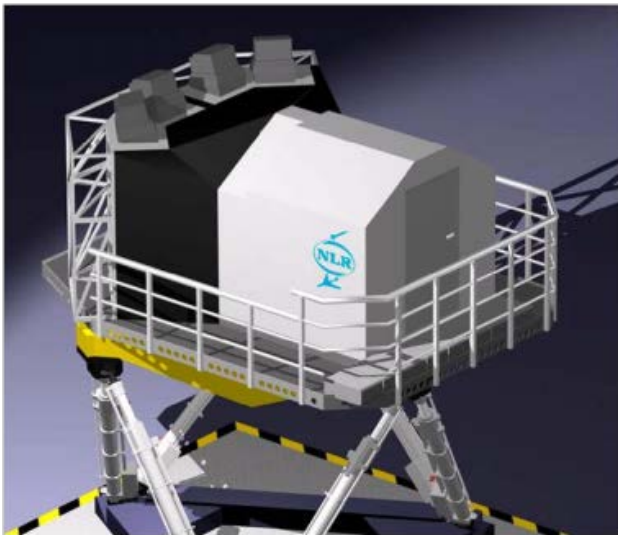
Figure 7: The Generic Research Aircraft Cockpit Environment (GRACE) at NLR, featuring a modifiable cockpit on a hexapod motion platform.
