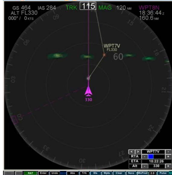
Fig. 1. A screenshot of the CSD and RAT. The weather scenario shown here is the Middle type.
