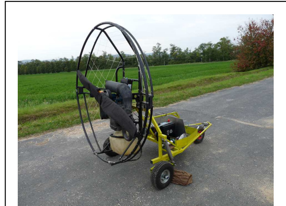
Fig. 4. The very first test of the PPG UAV developed on the department
