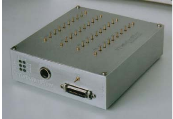
Fig. 3. Dynamic Pressure (DP) measurement module.
