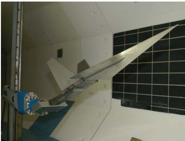
Fig. 1. View of the Generic Buffet Model in DSTO Low Speed Wind Tunnel.
