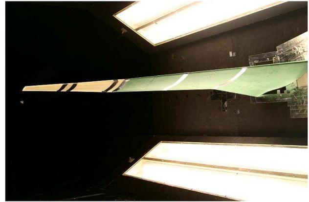
**Fig. 6** Planar wing model configuration in the wind tunnel.
