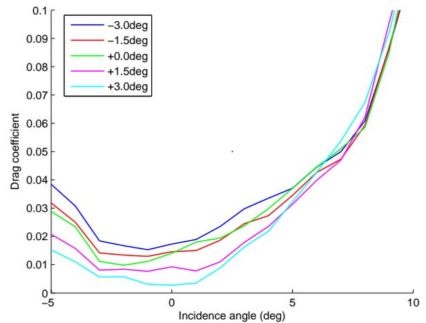
Fig. 9 Drag wind tunnel test results for varying twist angles.
