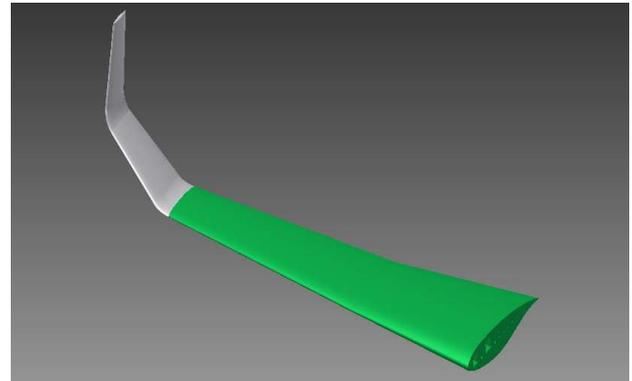
**Fig. 4** Planar wing CAD wind tunnel model design.
