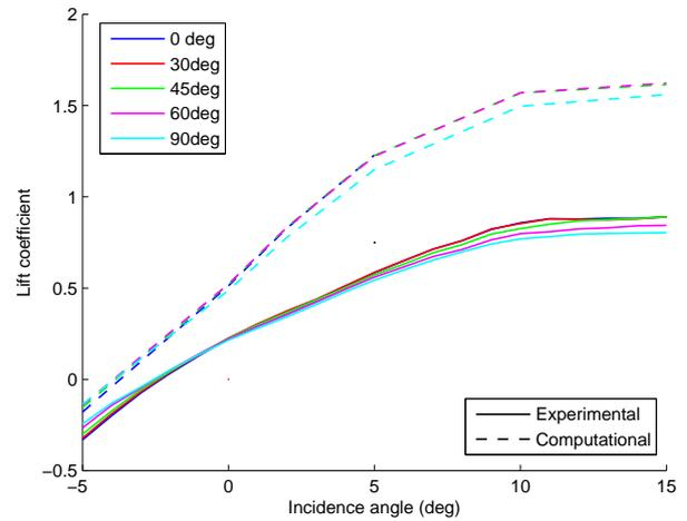
Fig. 8 Lift curve slope experimental and computational results for varying dihedral angles.
