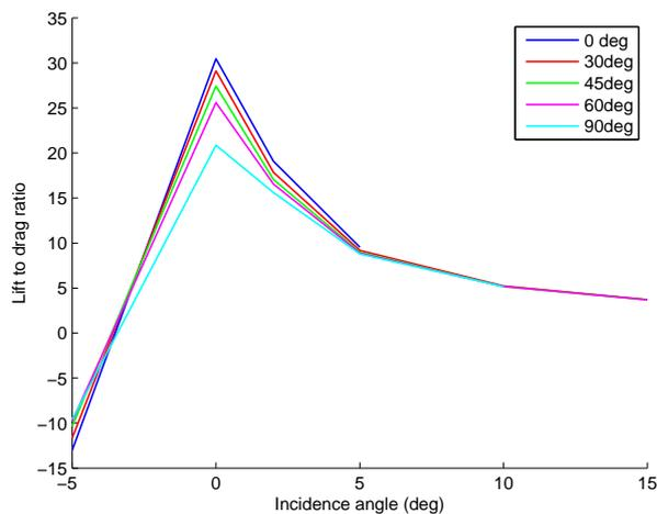
**Fig. 14** Lift to drag ratio for various dihedral angles, computational results.
