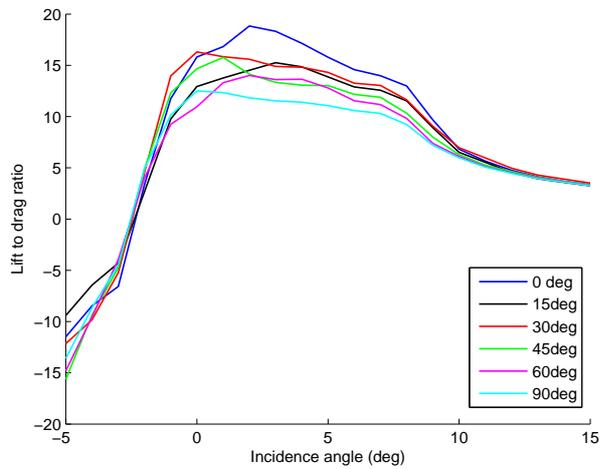
**Fig. 13** Lift to drag ratio for various dihedral angles, experimental results.
