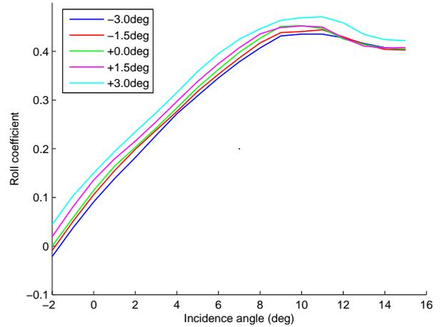
**Fig. 11** Experimental results for bending moment coefficient variation with incidence for varying twist.
