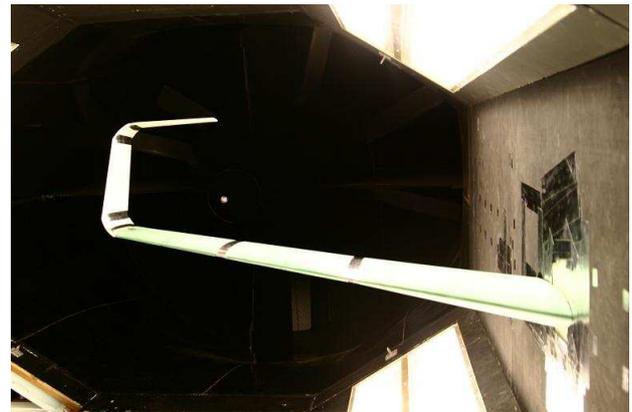
**Fig. 7** C-wing configuration in the wind tunnel.
