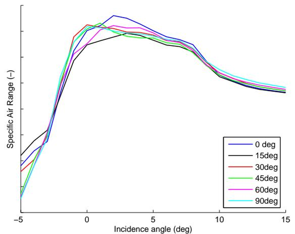
**Fig. 15** Specific range for various dihedral angles, wind tunnel results.
