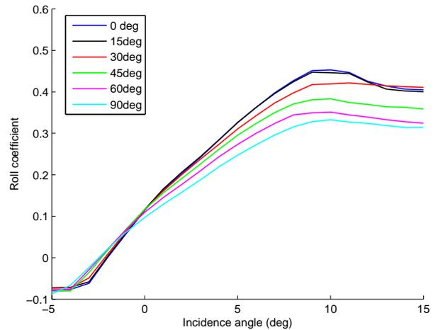
**Fig. 12** Experimental results for bending moment coefficient variation with incidence for varying dihedral.
