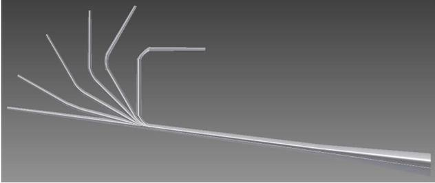
**Fig. 5** Demonstration of the ranges of dihedral variation for the wind tunnel model.
