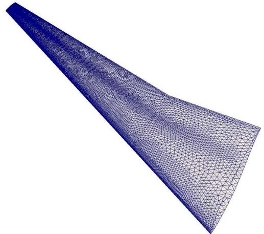
**Fig. 2** Planar wing mesh generated for Tau.
