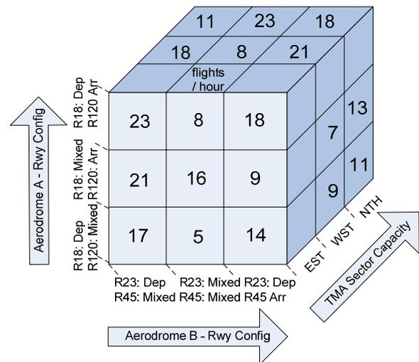
Figure 2: A multi-dimensional cube of gross differential capacities for TMA sectors.
