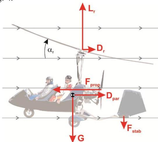
Fig. 4. Longitudinal and vertical forces acting on the gyroplane
