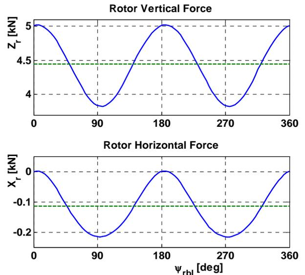
Fig. 9. MTOsport horizontal and vertical rotor forces at an airspeed of 65 kts
