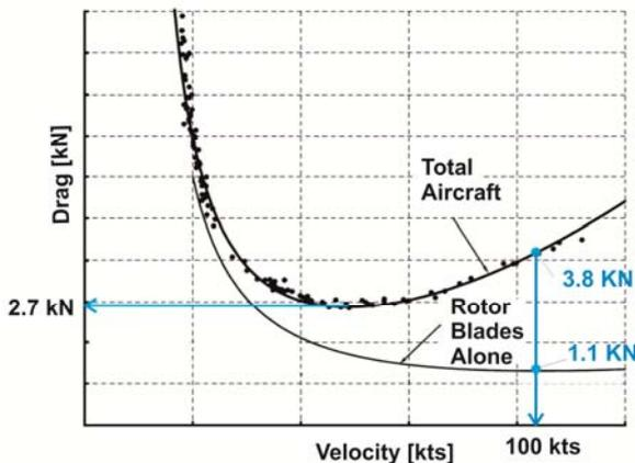
Fig. 6. PCA-2 gyroplane drag breakdown from gliding tests by Wheatley 1932 [5]
