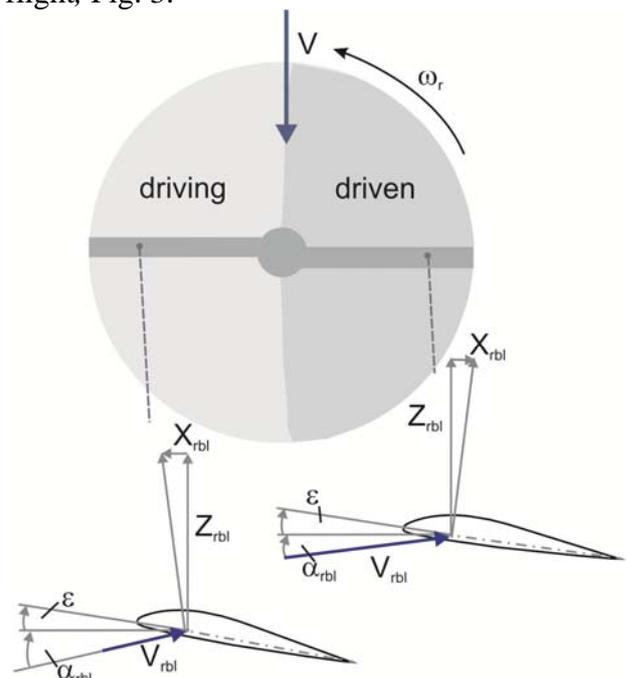
Fig. 3. Regions of driving and driven aerodynamic forces (forward flight)
