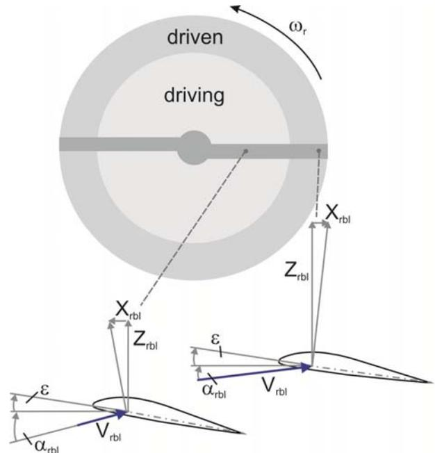
Fig. 2. Regions of driving and driven aerodynamic forces (vertical autorotation)
