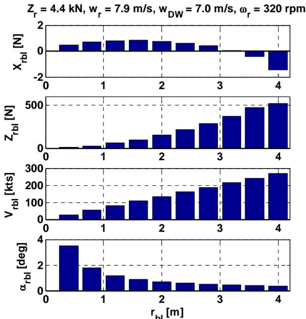
Fig. 8. MTOsport rotor forces during vertical autorotation (simulation)
