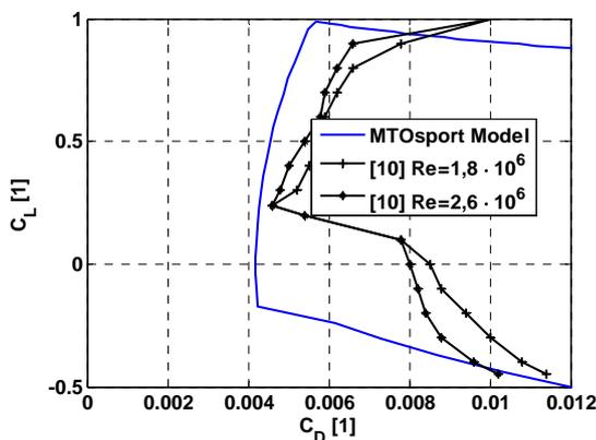
Fig. 7. Lift-drag polar of the NACA 8-H-12 airfoil from [10] and modified based on flight test data
