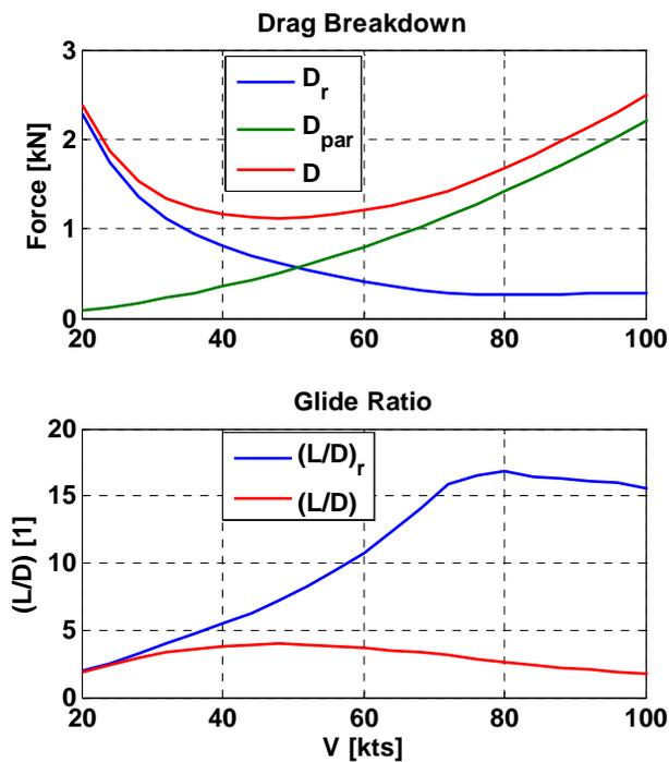
Fig. 10. MTOsport gyroplane drag breakdown and glide ratio (simulation)
