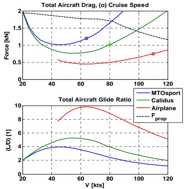
Fig. 12. Total aircraft drag and glide ratio over airspeed of MTOsport and Calidus gyroplanes and a generic light airplane (simulation)
