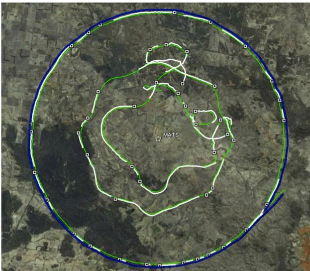
Fig. 5. Example flight test results of the MATS tracking the ASL. The figure shows radar tracks (white lines), the ASL's truth data (green lines) and the received ADS-B track of the ASL (blue line). The flight trial results are from tests performed at Burrandowan, Queensland.
