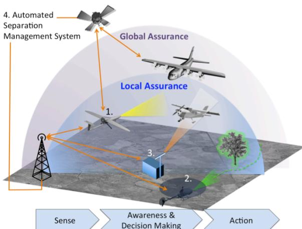
Fig. 1. Overview of Smart Skies technologies for separation management and collision avoidance
