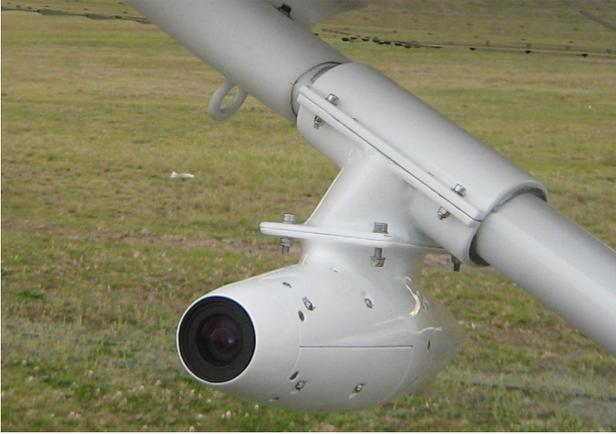
**Fig. 2** EO sensor pod mounted on wing support strut.
