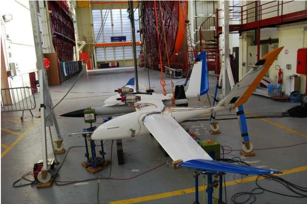
Fig. 9. EOLE Flutter Tests (Onera)
