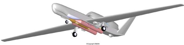
Fig. 3. Dedalus Phase II RQ-4 GlobalHawk Based Air-launch-to-orbit Concept with 3 parallel stage launcher
