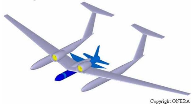
Fig. 1. Dedalus Phase I Air-launch-to-orbit Concept
