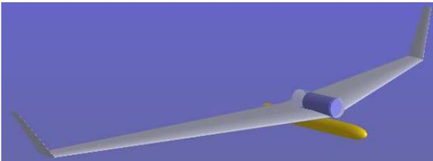
Fig. 6. L3AR Single-Engine Blended Wing Body Air-launch-to-orbit Concept
