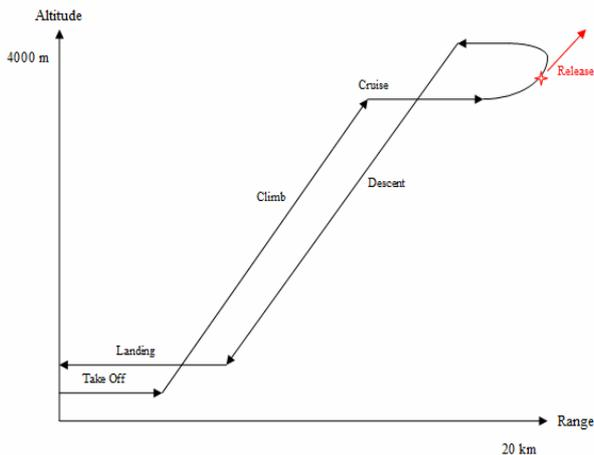
Fig. 12. Typical Air-launch-to-orbit Mission Profile (with 3g pull-up maneuver)
