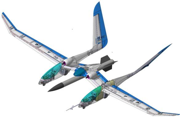
Fig. 8. CAD View of EOLE demonstrator with launcher
