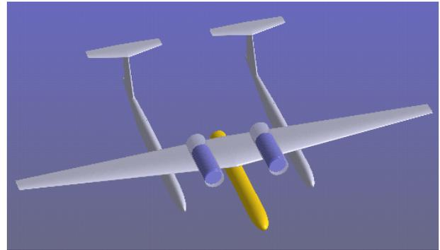
Fig. 4. Dedalus Phase II Nanosatellites Air-launch-to-orbit Concept
