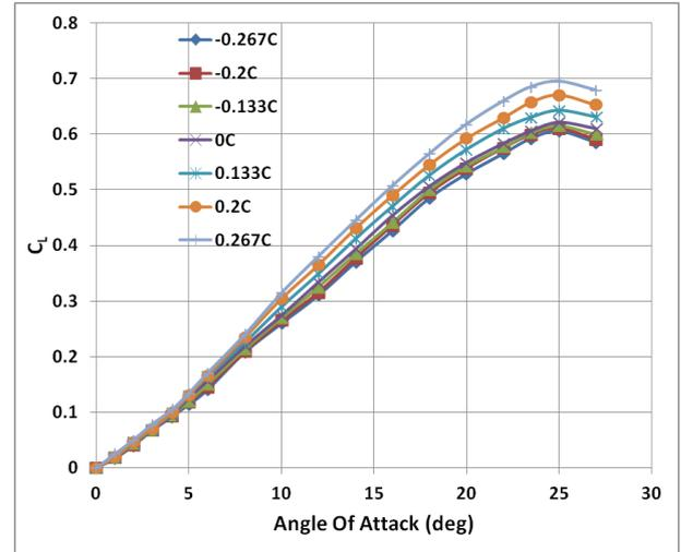
Fig. 5 Effect of Stagger on Lift at  $0.533\bar{c}$
