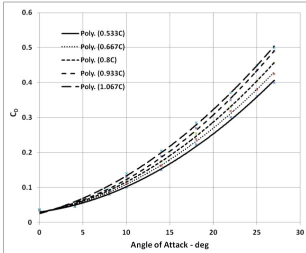
Fig. 11 Coefficient of Drag for various gap positions
