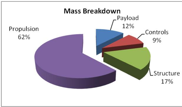
Fig. 13 Mass Breakdown of Black Widow MAV
