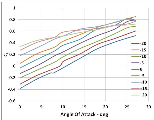
Fig. 8 Effect of Decalage angle at 1.067C gap and zero stagger
