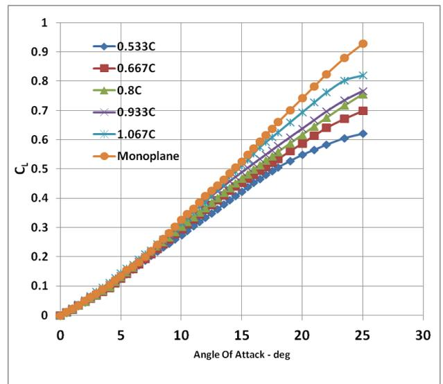
Fig. 10 Coefficient of Lift for various gap positions
