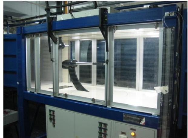
Fig. 3 Closed-circuit wind-tunnel test section with sting balance
