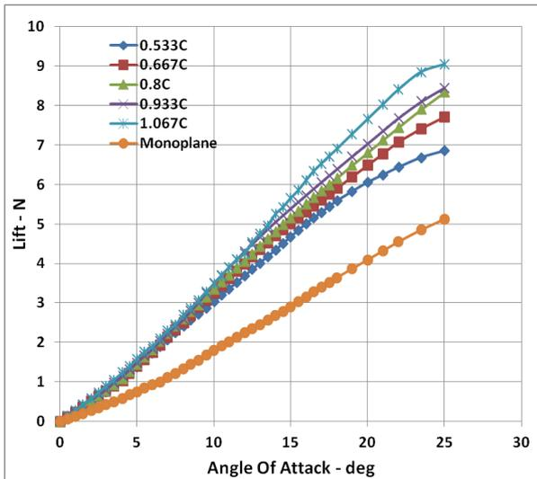
Fig. 4 Lift of monoplane and biplanes (various gaps)
