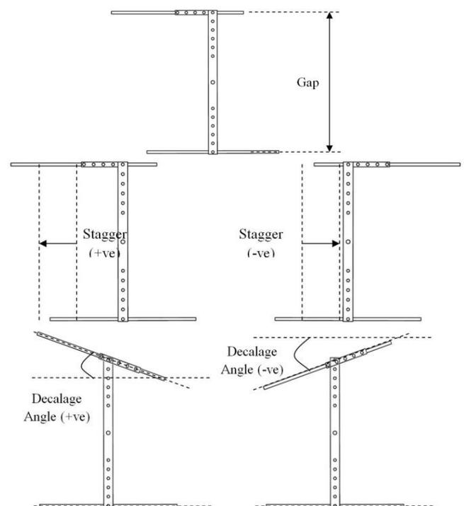
Fig. 1 Geometric attributes: Gap, Stagger and Decalage angle
