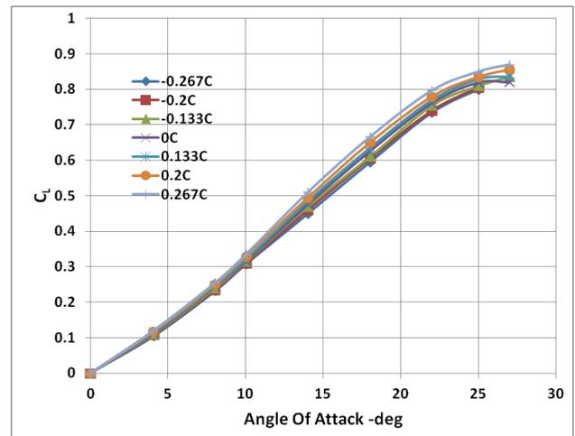
Fig. 6 Effect of Stagger on Lift at  $1.067\bar{c}$
