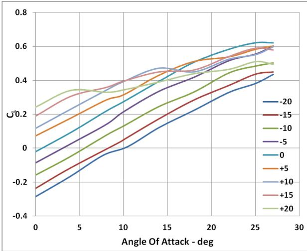
Fig. 7 Effect of Decalage Angle at 0.533C gap and zero stagger
