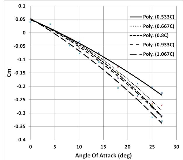
Fig. 12 Coefficient of pitching moment for various gap positions
