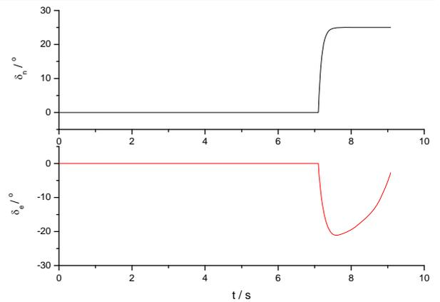
Fig. 3 Control effector deflections without TV during ground run
