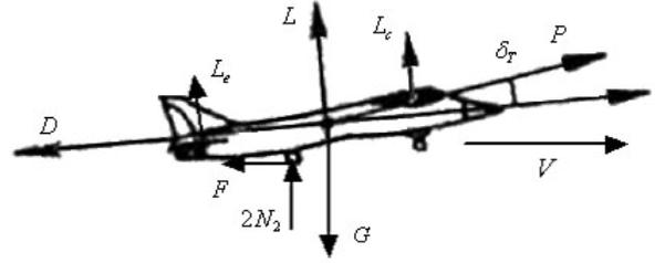
Fig. 1 Force acting on aircraft with TV during takeoff ground run
