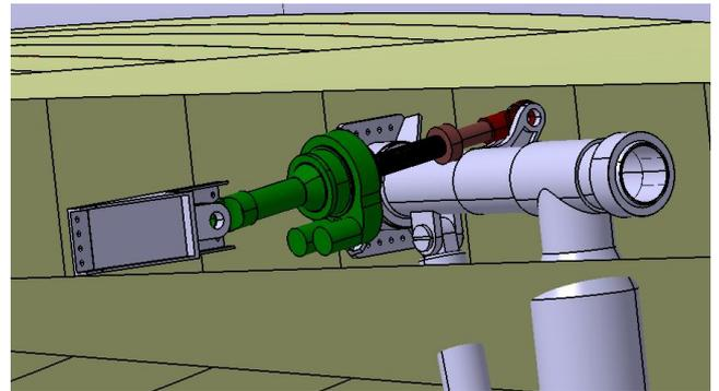
Fig.8. EMA installation-landing gear lowered
