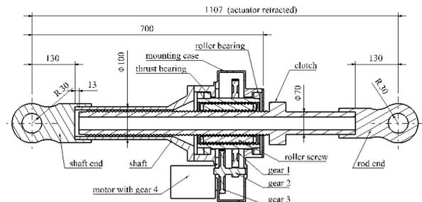
Fig.2.EMA cross section view
