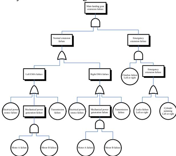
Fig.10.Fault tree analysis
