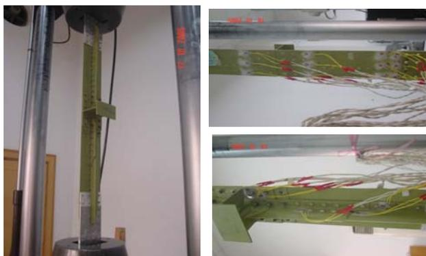
**Stringer fitting fatigue test**
