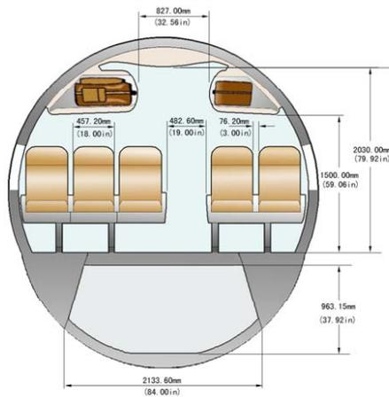
Diagram illustrating the Cabin Cross Section of the ARJ21-700, showing dimensions in millimeters (mm) and inches (in):
