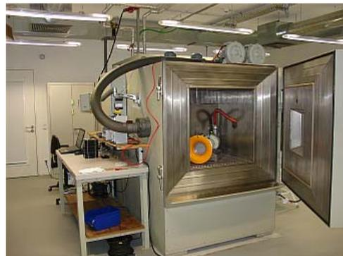
Fig. 14. Flowmeter to measure pressure drop across porous surfaces and metering orifices; measurements are performed in a climate chamber
