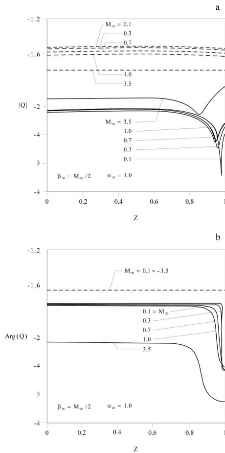
**Fig. 5** As Figure 4, with the relation  $\beta_\infty = M_\infty/2$  to ensure that there is a critical level in the middle of the boundary layer  $y_c = L/2$ .
