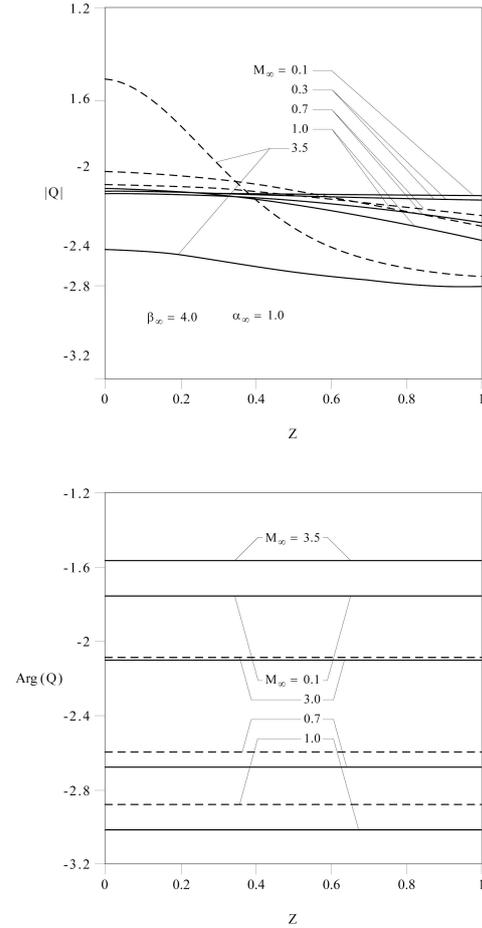
**Fig. 4** As Figure 1, comparing the sound fields due to a line source for homenergetic (solid line) and homentropic (dotted line) shear flows, for low speed  $M_\infty = 0.1$ , incompressible  $M_\infty = 0.3$ , subsonic  $M_\infty = 0.7$ , sonic  $M_\infty = 1$  and supersonic  $M_\infty = 3.5$  free streams. Wave frequency equal to vorticity  $\alpha_\infty = 1$  and  $\beta_\infty = 4$
