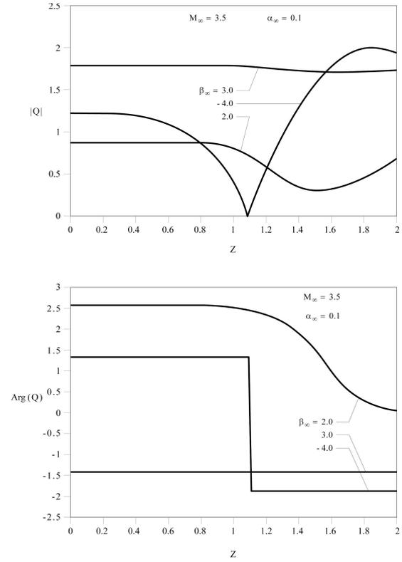
**Fig. 3** As Figure 1, for supersonic free stream  $M_\infty = 3.5$ , wave frequency much smaller than vorticity  $\alpha_\infty = 0.1$ , and three values of  $\beta_\infty$ .
