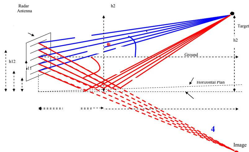
The figure 3 below represents an example of elevation measurement disturbance due to the multi path effects in a standard radar signal processing along the range.
