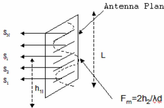
Figure 6 Shape of the received recombined signal on antenna surface.
