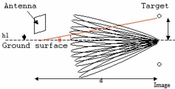
Figure 5 Recombined signal received on the antenna
