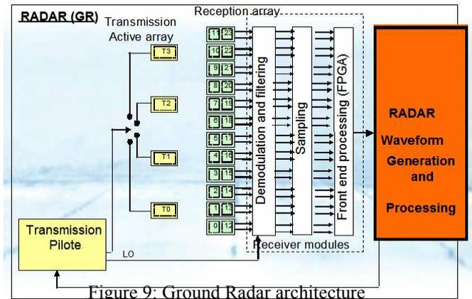
Figure 9: Ground Radar architecture
