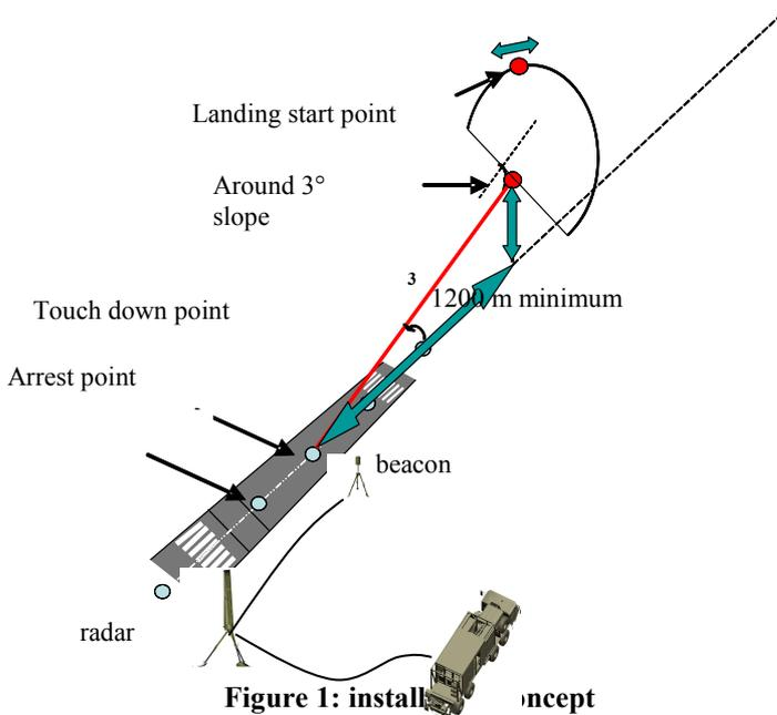
Figure 1: installation concept
