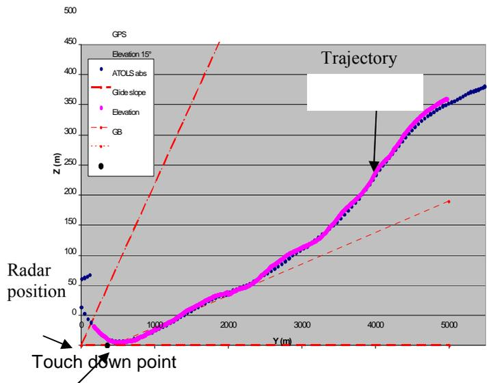
Figure10: Elevation measurement: height versus range
