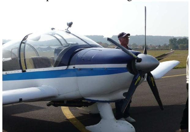
Fig. 15 DR400 equipped with ANIBAL propeller
