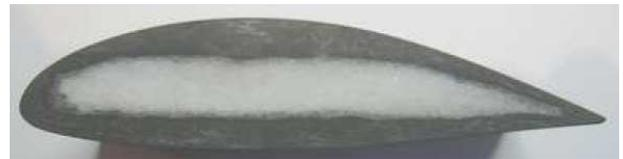
**Fig. 4 Overview of blade internal structure (composite technology)**
