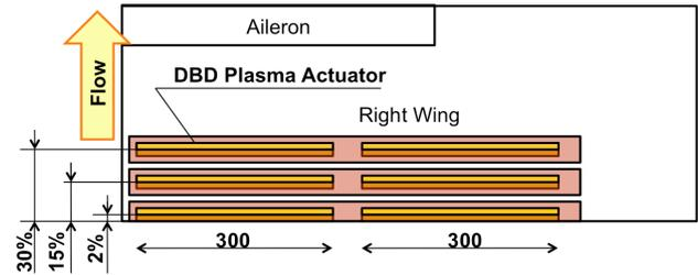
**Fig. 4** Location of DBD plasma actuator on the main wing
