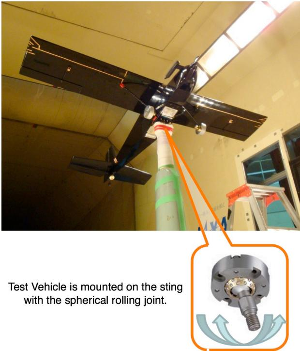
Test Vehicle is mounted on the sting with the spherical rolling joint.
