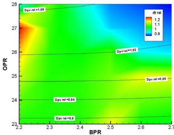
Fig. 2. Influence of  $OPR$  and  $BPR$  on emission parameters  $D_{pv,rel}$  and  $dt_{rel}$ .
