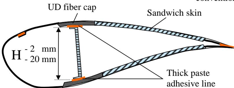
Fig. 9: Turbine Blade – Typical Design
