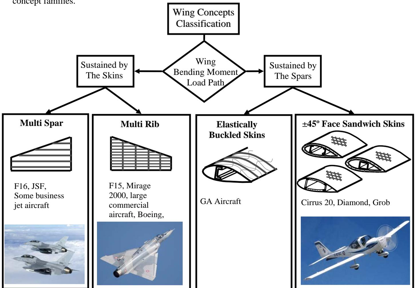
*Fig.1: Wing Structure Classification*
