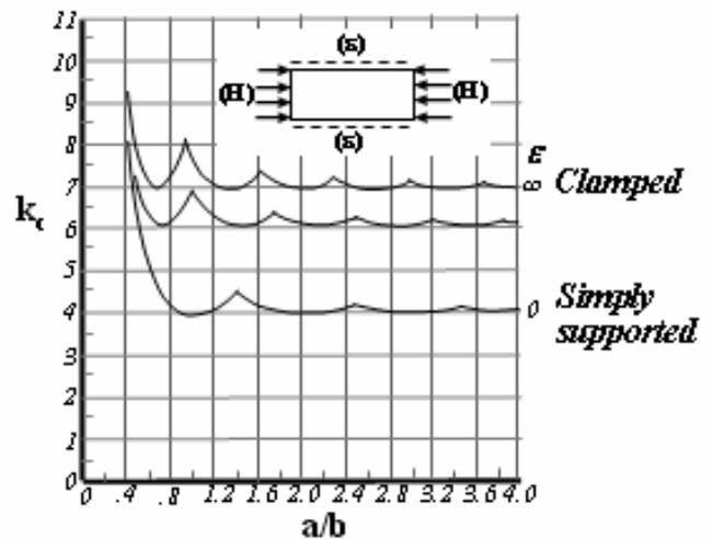
*k<sub>c</sub>, Coefficients with various edge rotational restraints (Compression).*
