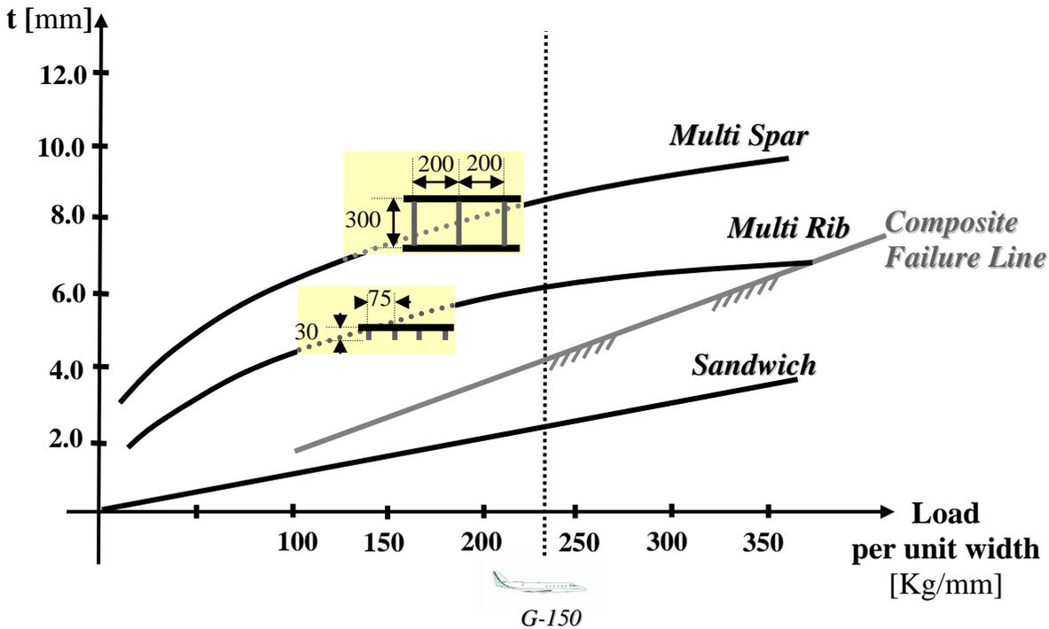
Fig. 8: Load – Thickness Curves for Composites
