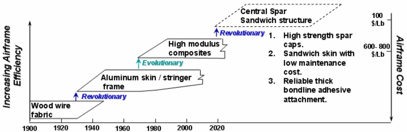
Fig. 11: Revolutionary versus Evolutionary Design Advancement of Airframe Structures
