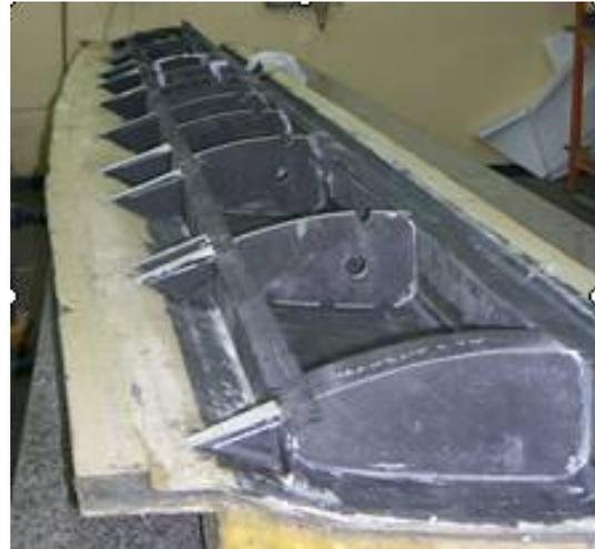
Fig. 6: Wing Ribs with Fuel Passages
