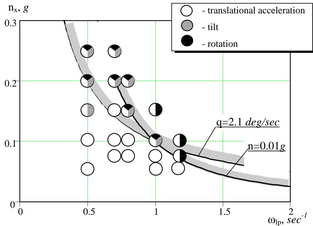
Fig.10. The boundaries of false sensations arising during low-frequency longitudinal accelerations simulation.
