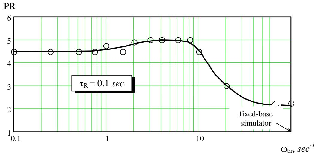
Fig.4. The influence of washout filter break frequency on motion fidelity for negative acceleration effect.
