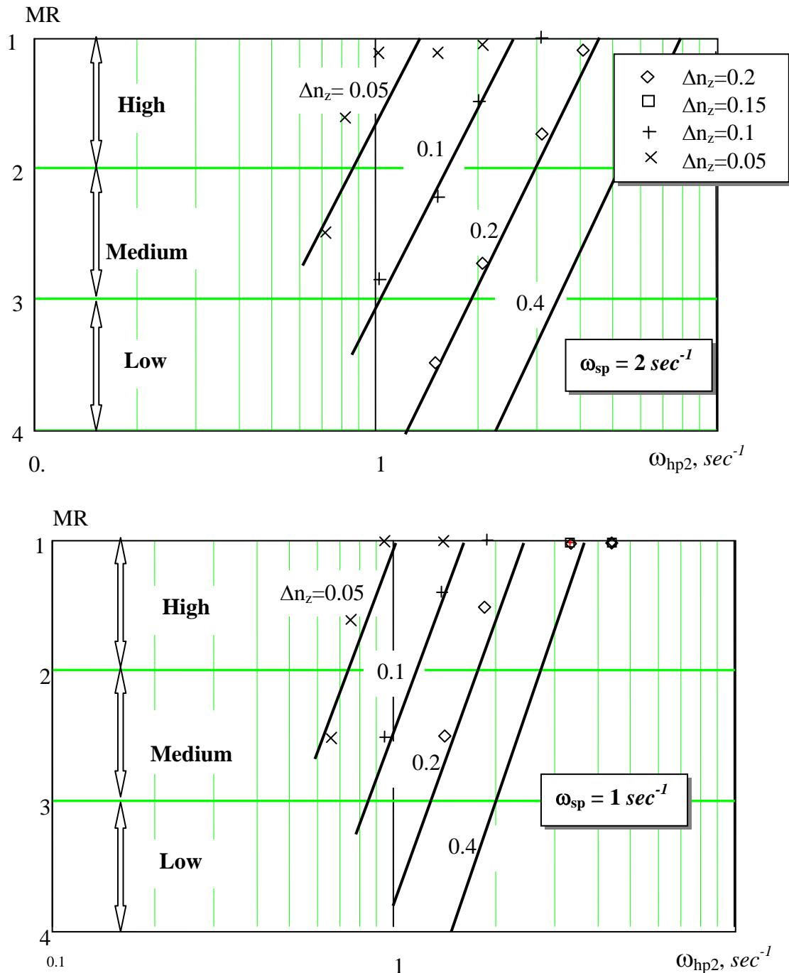
Fig.7. Simulation fidelity for rear edge of normal accelerations vs 2<sup>nd</sup> order filter frequencies, for different short-period mode frequencies.
