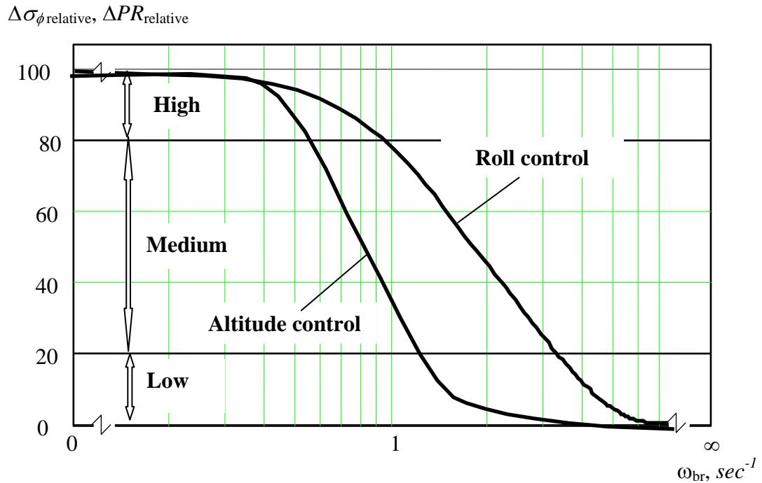
Fig.1. Motion fidelity as a function of high-pass filter break frequency for precision control tasks. Beneficial acceleration effect.
