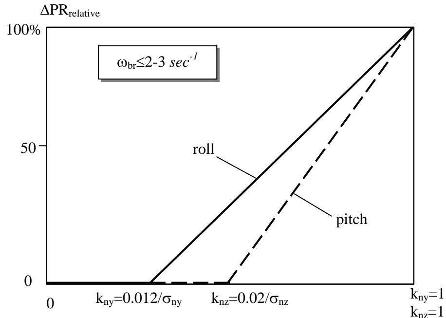
Fig.5. A criterion to estimate the influence of scaling for negative acceleration effect.
