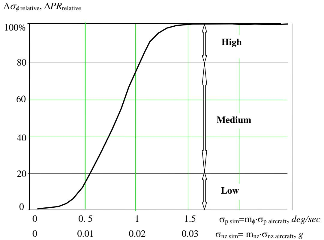
Fig.3. Motion fidelity as a function of simulator roll rate RMS and normal accelerations RMS.
