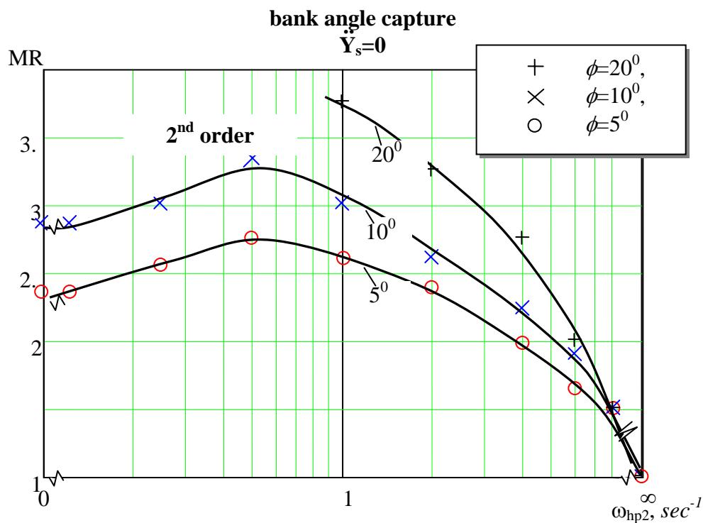
Fig.9. Integrated effects of false lateral accelerations and false opposite roll rates on motion fidelity ratings; the 2<sup>nd</sup> order high-pass filter.
