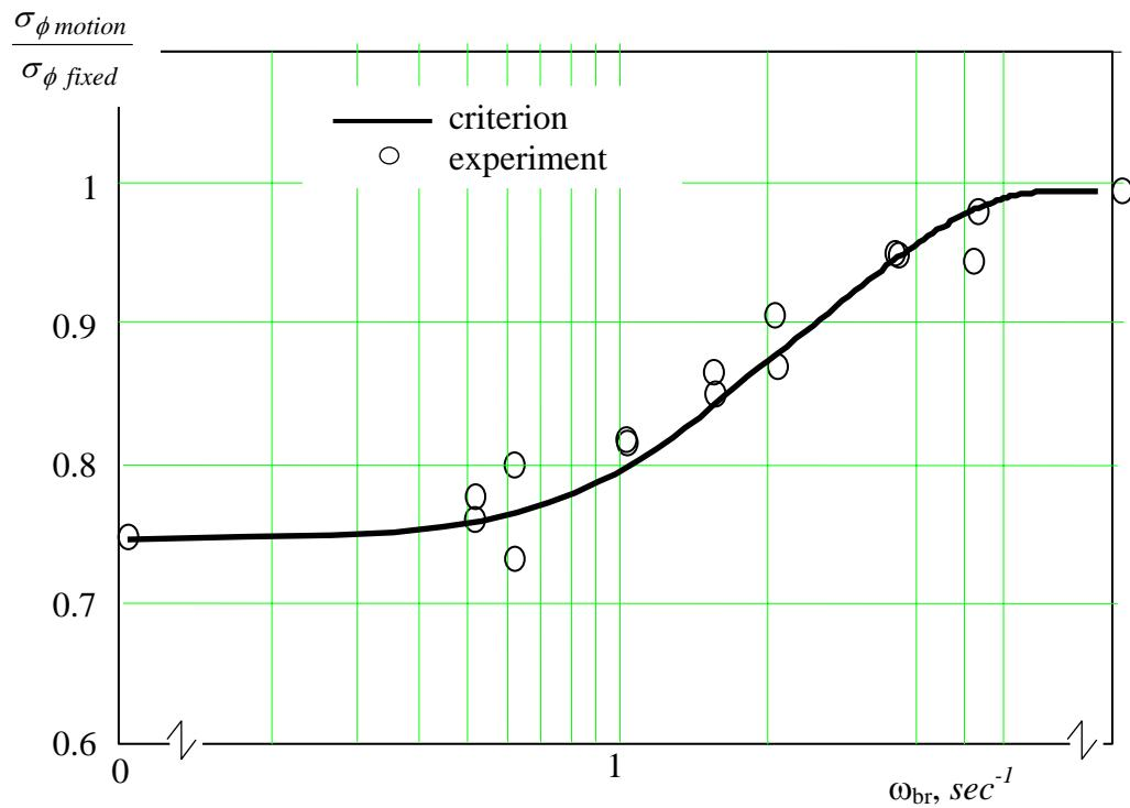
Fig.2. Example of the experimental data received on the criterion for high-pass filtering. Roll control task. Beneficial acceleration effect.
