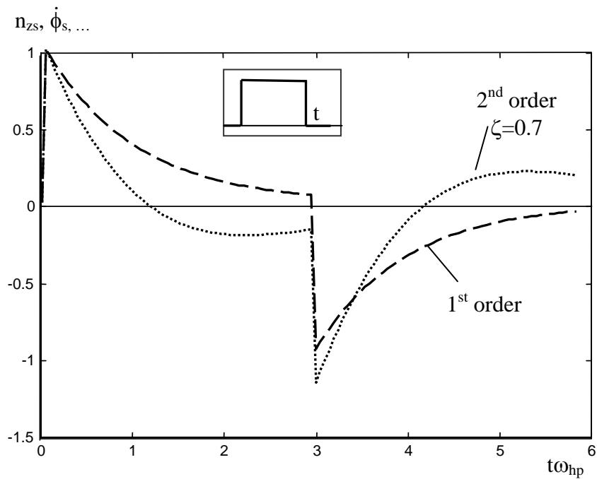
Fig.6. High-pass filters response to square-type input.
