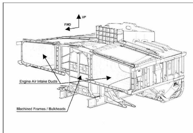
Fig. 7-1 Typ. center fuselage structure (outer skin panels not shown)
