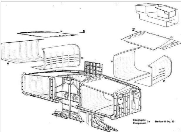
Fig. 3.1 TORNADO Center Fuselage structure
