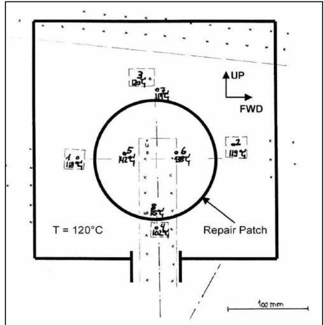
Fig. 7.2-4 Heat sensor elements during simulated bondline curing
