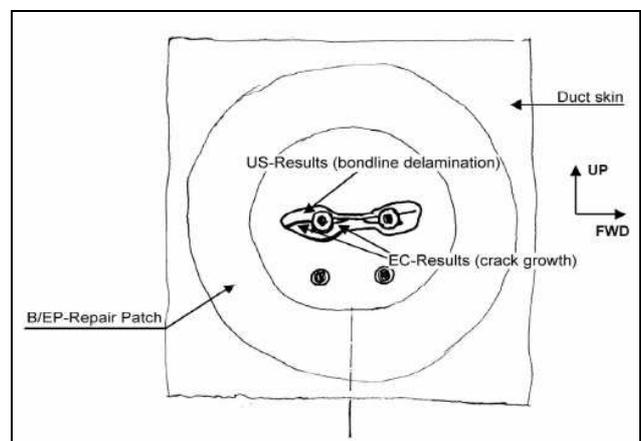
Fig. 7.3-2 EC-NDI Results at 1000 testhours
