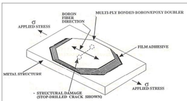
Fig.4-1 Bonded composite patch (typ.)
