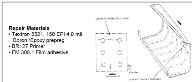
Fig 7-2 Repair location in engine duct
