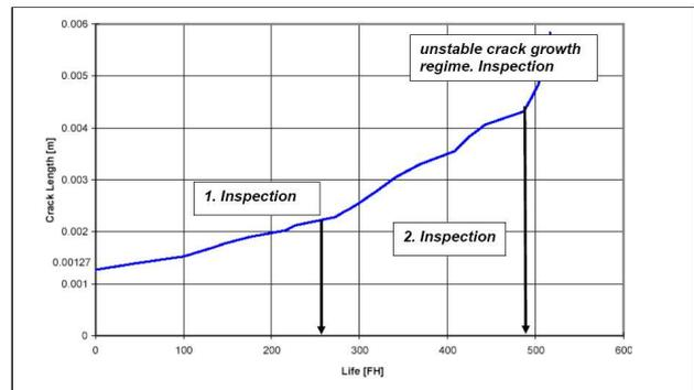
Fig. 3.3 Typ. Crack growth in AL 7075 components at high stress level and crack intensity factors
