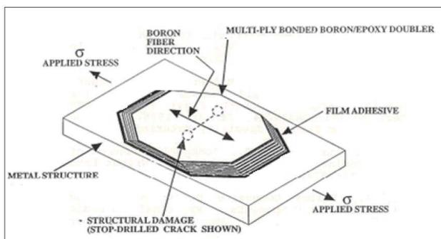
Fig.4-1 Bonded composite patch (typ.)
