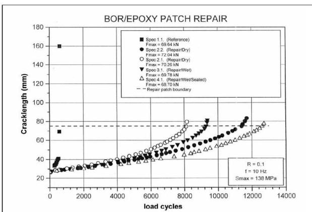
Fig. 6.6-1 Component Tests (Const. Amplitude)
