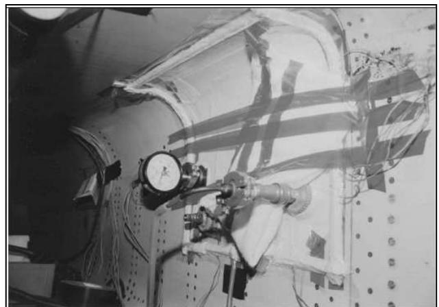
Fig. 7.2-5 Repair bonding process
