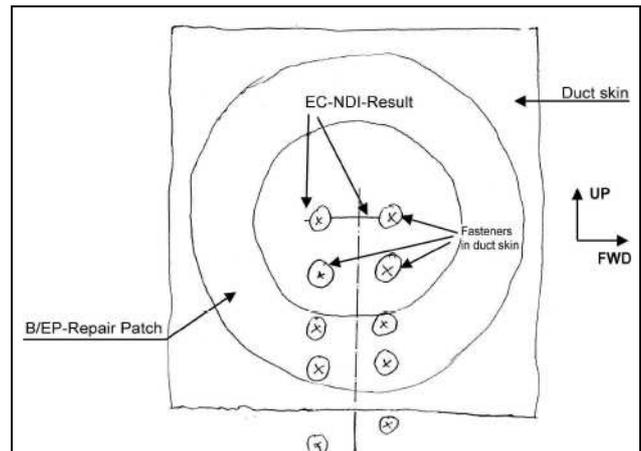
Fig. 7.3-1 EC-NDI Results at 500 Testhours
