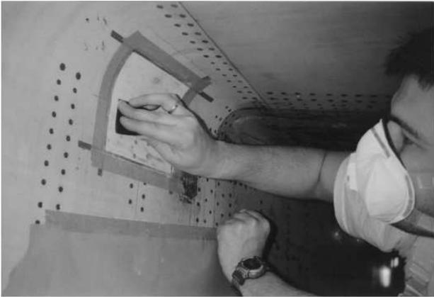
Fig. 7.2-2 Surface preparation in repair zone
