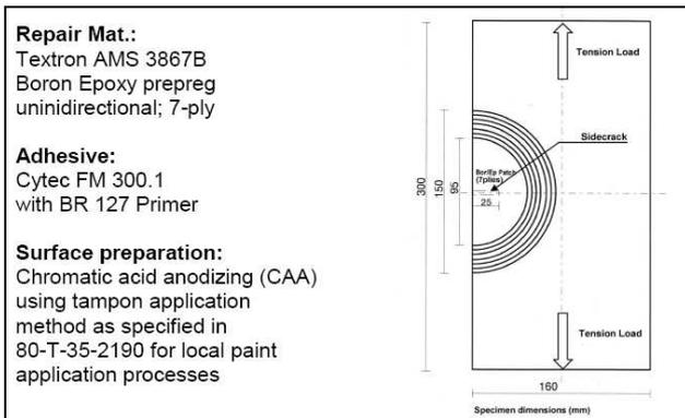
Fig. 6.4-1 "Single side" Crack Tension Specimen
