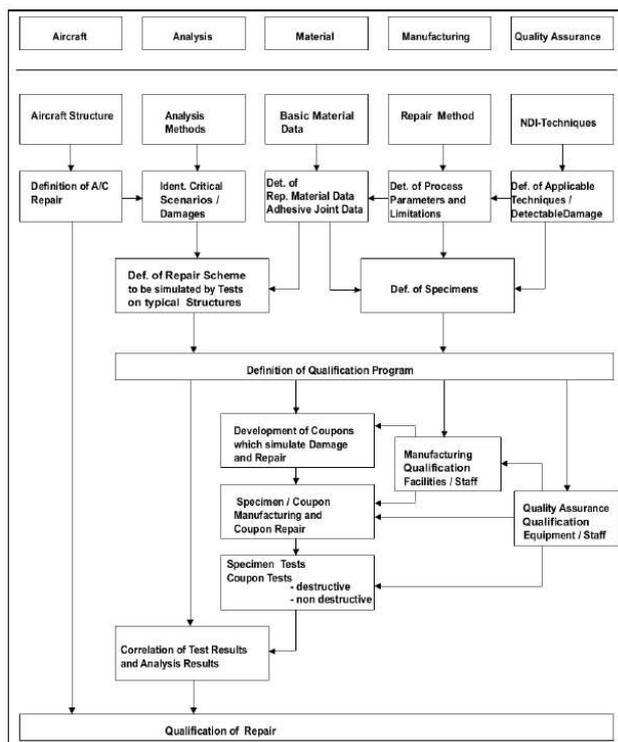
Fig 6-1 Route to Qualification of A/C- repairs
