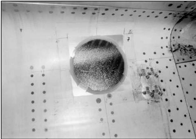
Fig. 7.2-6 Repair bonded to duct skin
