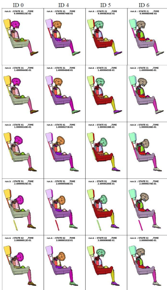
Fig. 7 Flight Helmet HMD- Hybrid III Head motion ID 0, ID4, ID5 and ID6
