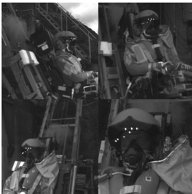
Fig 3. Qualification test with Daycamera and QRC separation.
