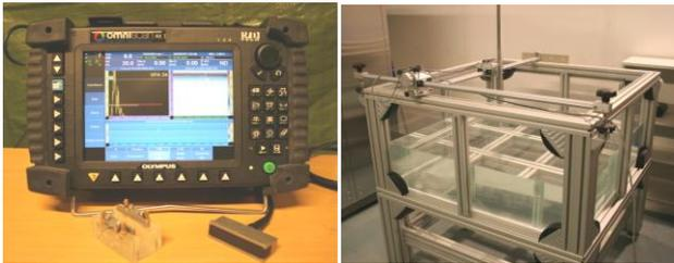
Fig. 4. Ultrasonic NDI equipment (left) and water tank with xy-scanner (right)
