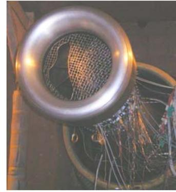
*Fig. 5. Fan intake duct with the mounted flow non-uniformity simulator*
