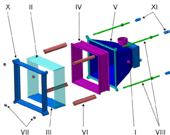
**Fig. 3: Combustion chamber**
