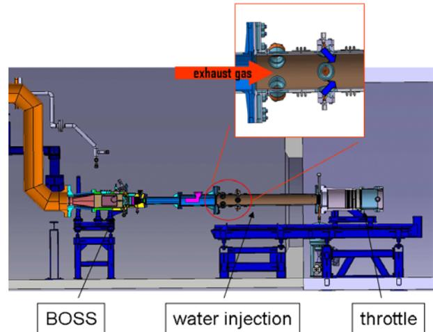
**Fig. 7: Water injection and throttle at HBK1**
