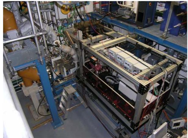
**Fig. 9: Container with planar measurement techniques hardware at the test section**
