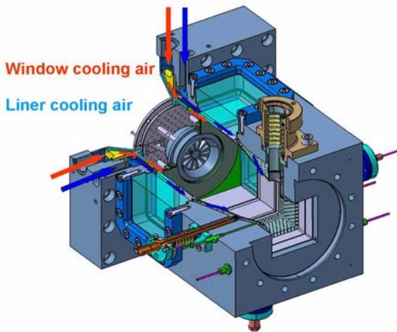
**Fig. 5: Cooling setup**
