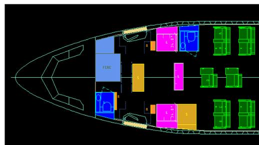
Fig. 1 Cabin layout obtained with Pacelab Cabin tool
