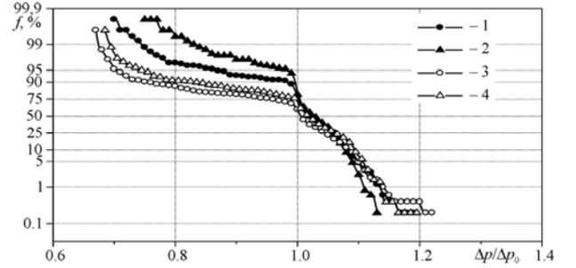
Fig. 4. Cumulative probability  $f$  of  $\Delta p/\Delta p_0$  in the sonic boom wave propagating through stochastic field.
