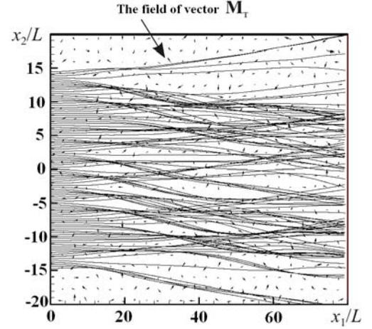
Fig. 3. Propagation of the acoustic rays through the random velocity fluctuations field.
