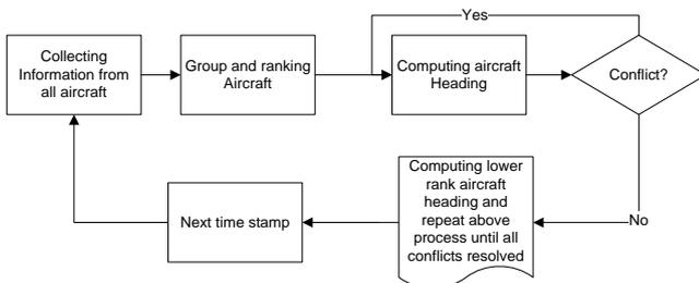
Figure 2: Process of Delay based Ranking Separation Algorithm
