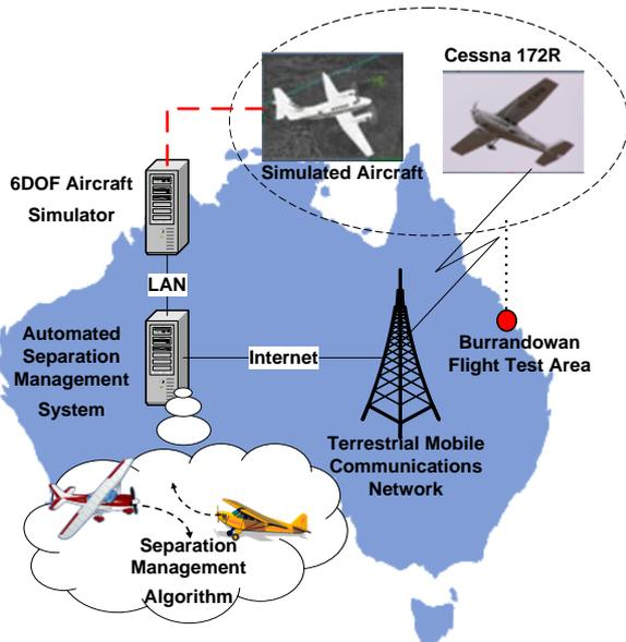
Figure 7: The automated separation management system architecture
