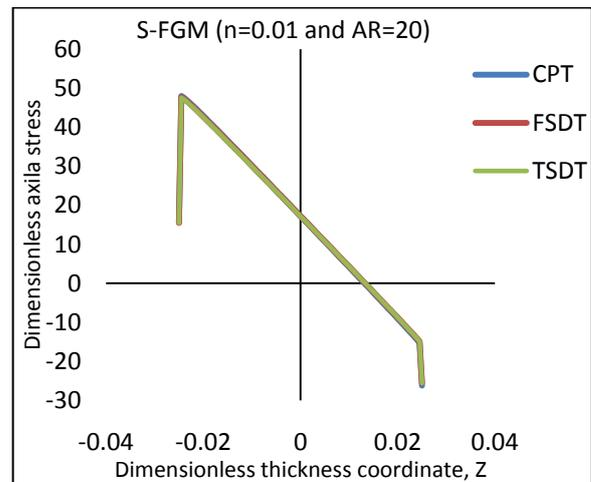
Fig. 6.  $\sigma$  at the center of the plate under load  $Q=-400$  for  $AR=20$  in S-FGM plate
