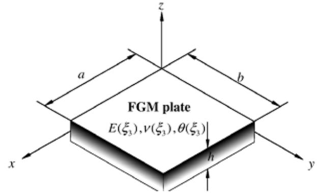
Fig. 1. Geometry of FGM plate
