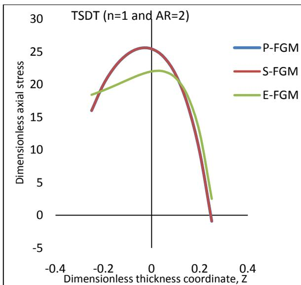
Fig. 16. Comparison of axial stresses for P-FGM, S-FGM and E-FGM based on TSDT
