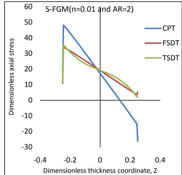
Fig. 8.  $\sigma$  at the center of the plate under load  $Q=-400$  for AR=2 in S-FGM plate
