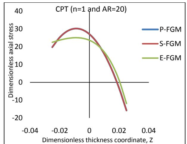
Fig. 13. Comparison of axial stresses for P-FGM, S-FGM and E-FGM based on CPT
