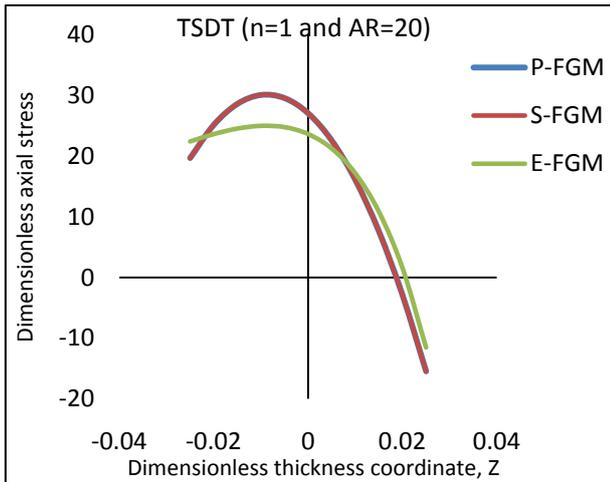
Fig. 14. Comparison of axial stresses for P-FGM, S-FGM and E-FGM based on TSDT
