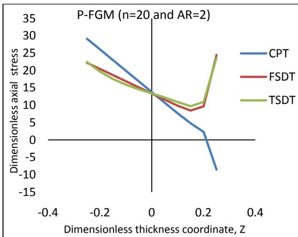
Fig. 11.  $\sigma$  at the center of the plate under load  $Q=-400$  for  $AR=2$  in P-FGM plate
