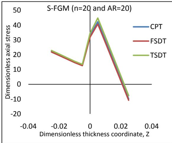
Fig. 10.  $\sigma$  of the plate under load  $Q=-400$  for  $AR=20$  in S-FGM plate
