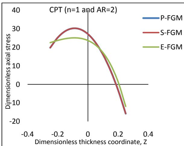
Fig. 15. Comparison of axial stresses for P-FGM, S-FGM and E-FGM based on CPT
