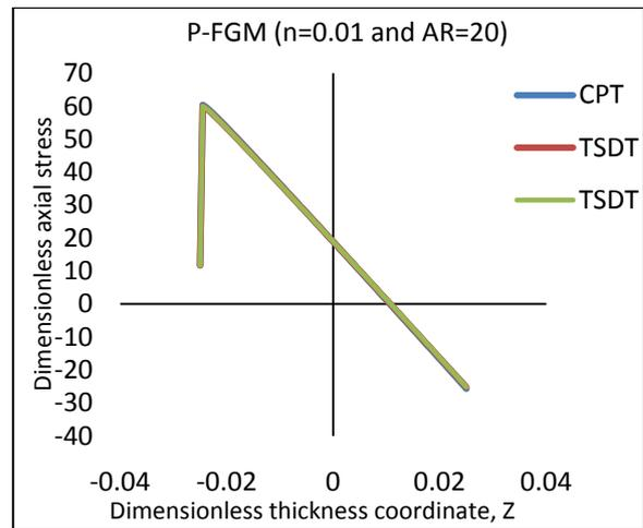
Fig. 5.  $\sigma$  at the center of the plate under load  $Q=-400$  for  $AR=20$  in P-FGM plate
