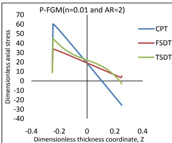
Fig. 7.  $\sigma$  at the center of the plate under load  $Q=-400$  for AR=2 in P-FGM plate
