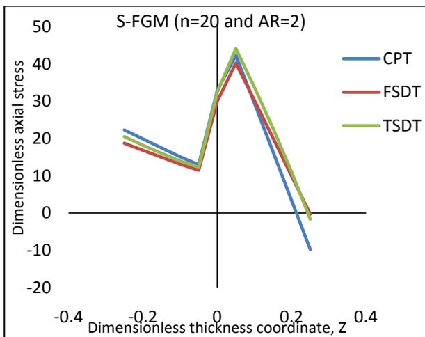
Fig. 12.  $\sigma$  at the center of the plate under load  $Q=-400$  for  $AR=2$  in S-FGM plate
