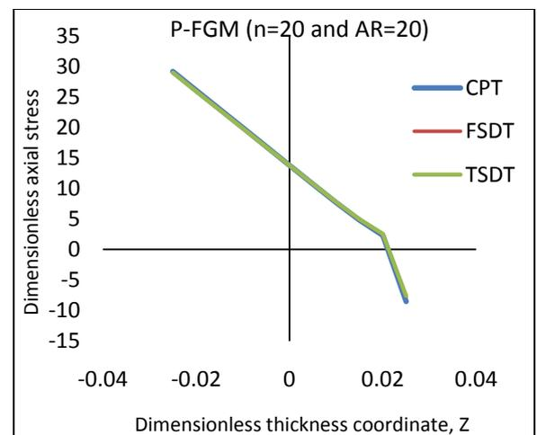
Fig. 9.  $\sigma$  at the center of the plate under load  $Q=-400$  for AR=20 in P-FGM plate
