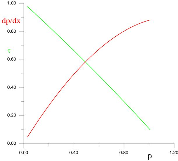
**Fig. 3.** Induced pressure gradient and skin friction distributions as functions of induced pressure for  $\beta = 0.75$
