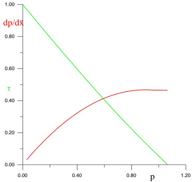
**Fig. 1.** Induced pressure gradient and skin friction distributions as functions of induced pressure for  $\beta = 0.25$
