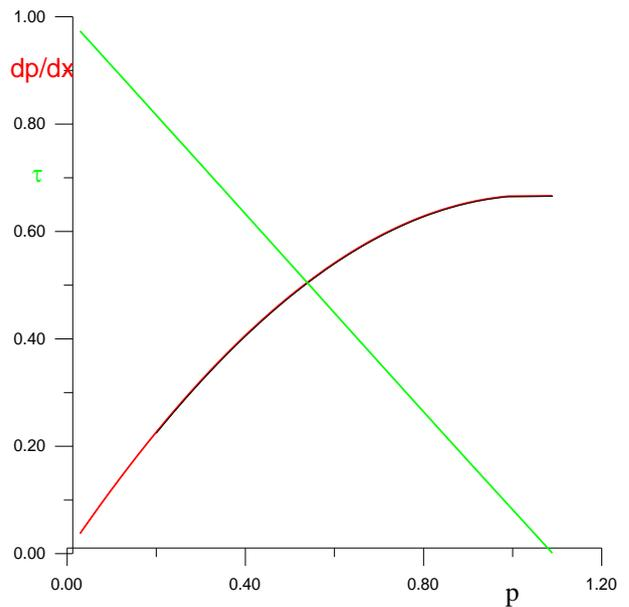
**Fig. 2.** Induced pressure gradient and skin friction distributions as functions of induced pressure for  $\beta = 0.50$
