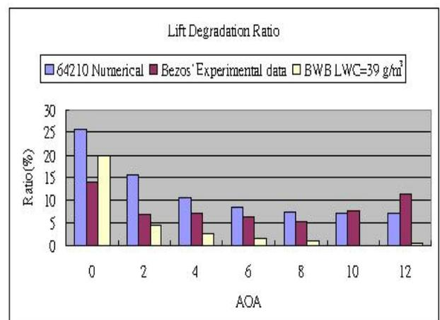
Fig. 10 Lift degradation comparison of BWB with NACA64-210 numerical and Bezos' data ( $LWC=39\text{g/m}^3$ )
