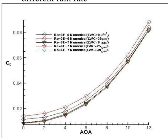
Fig. 9 BWB drag coefficients comparison for different rain rates
