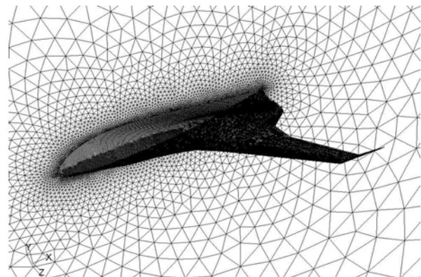
Figure 5 Near mesh of the Blended-Wing-Body
