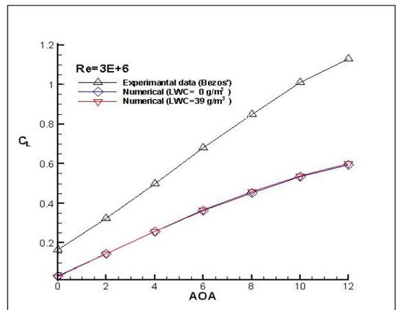
Fig. 6 Lift coefficients for 2 numerical results comparing to experiment data
