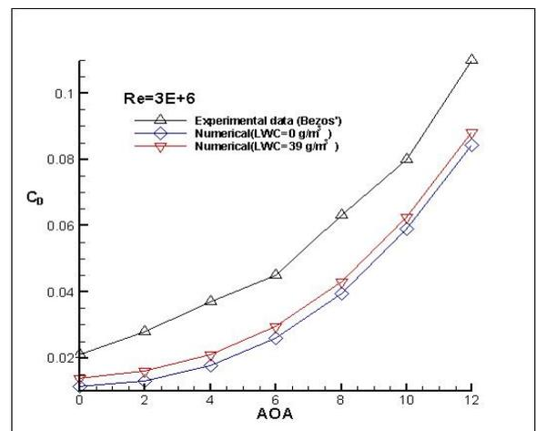
Fig. 7 Drag coefficients for 2 numerical results comparing to experiment data
