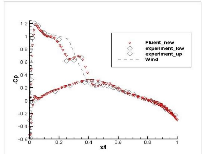
Fig. 2 Pressure coefficients on the wing surface at section  $(y/b)=0.80$
