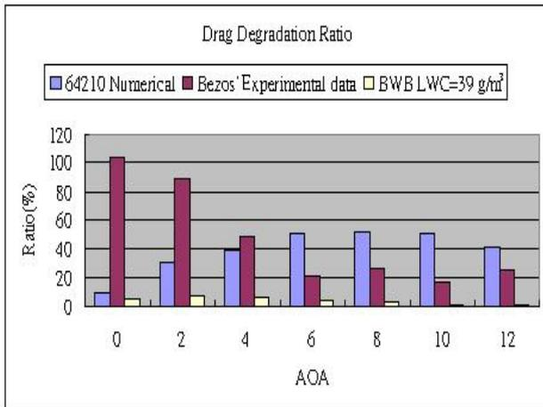
Fig. 11 Drag degradation comparison of BWB with NACA64-210 numerical and Bezos' data (LWC=39g/m<sup>3</sup>)
