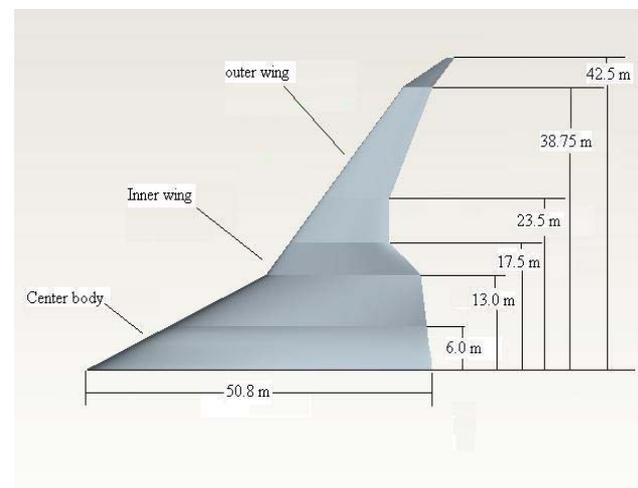
Fig. 1 Blended-Wing-Body geometry model
