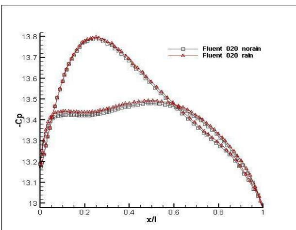
Fig. 13 Pressure coefficients on the wing surface at section (y/b)=0.20
