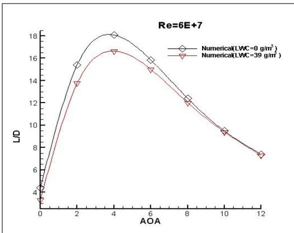
Fig. 12 Lift-to-Drag ratio change due to rain
