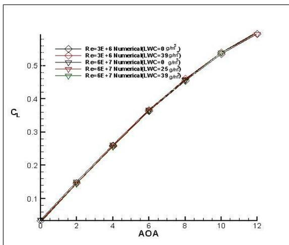
Fig. 8 BWB lift coefficients comparison for different rain rate
