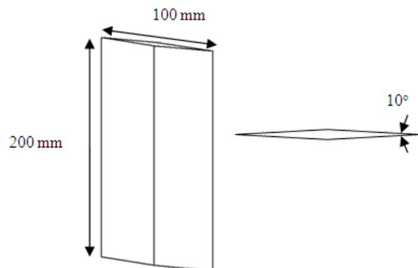
Fig 2. Geometry of Conventional Fin
