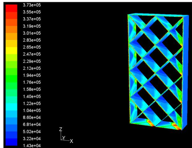
Fig. 5. Pressure Contours at  $M=2.5$  and  $10^\circ$  AOA
