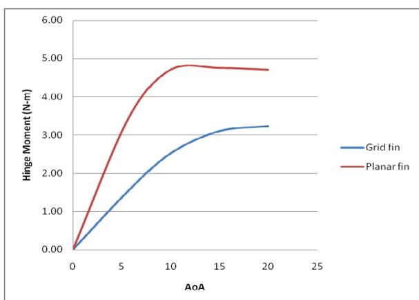
Fig. 6. Hinge Moment Vs AOA variation at M=0.5
