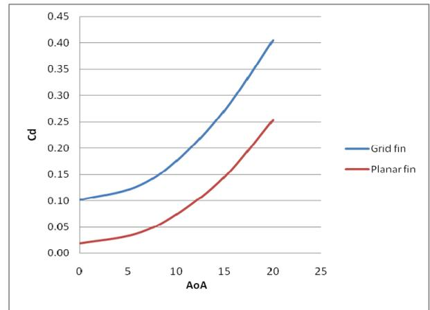
Fig. 10.  $C_d$  Vs AoA variation at  $M=2.5$
