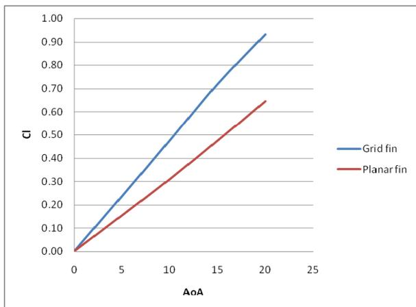
Fig. 10.  $C_l$  Vs AoA variation at  $M=2.5$
