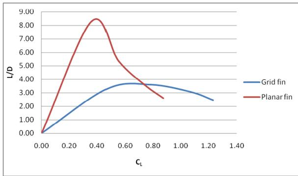
Fig. 8. L/D Vs  $C_L$  variation at  $M=0.5$
