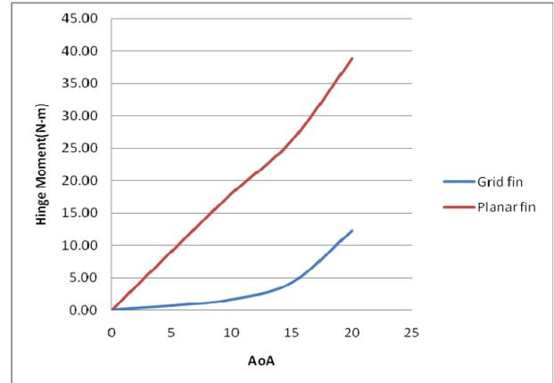
Fig. 7. Hinge Moment Vs AOA variation at M=2.5
