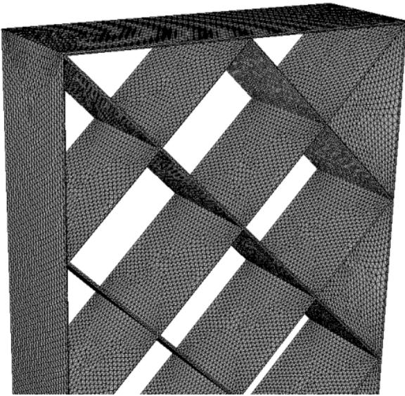
Fig. 3. Mesh Generated on the Grid Fin Surface
