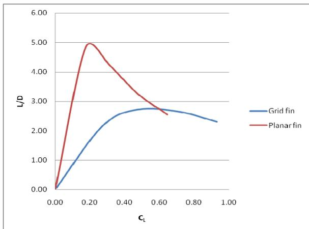
Fig. 9. L/D Vs  $C_L$  variation at  $M=2.5$
