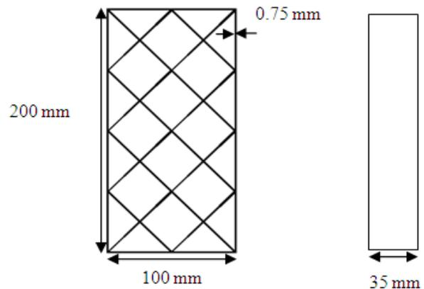
Fig. 1. Geometry of Grid Fin
