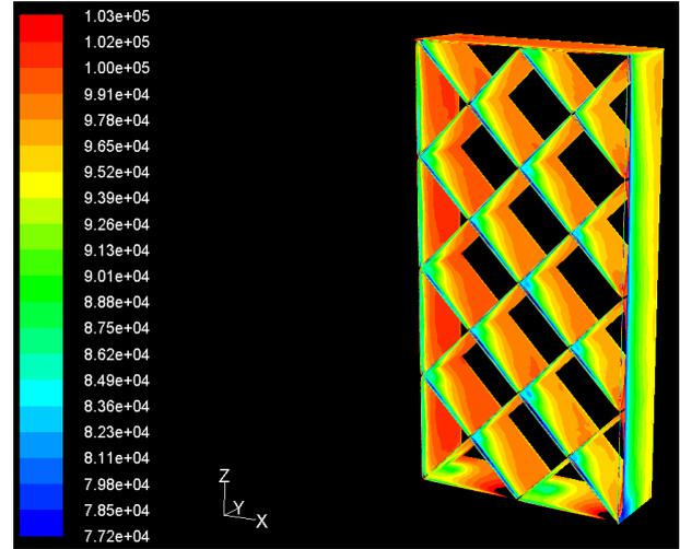
Fig. 4. Pressure Contours at  $M=0.5$  and  $10^\circ$  AOA
