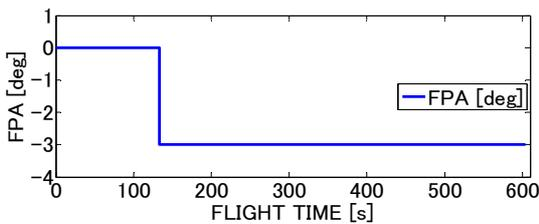
Fig. 6 Flight path angle- sample descent trajectory
