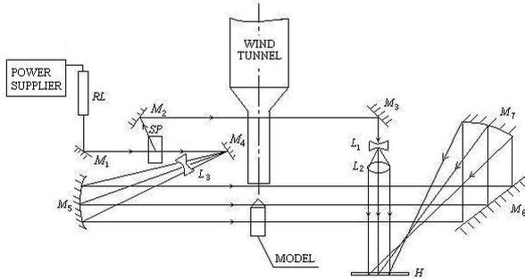
Fig. 1. The diagram of dual hologram interferometry optical system
