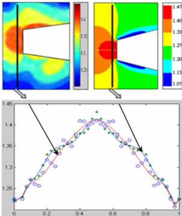
Fig. 12. The comparison of the density distribution (Red line with o indicates the experimental result. Blue line with \* indicates the numerical simulation result.)
