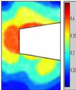
Fig. 9. The density distribution of the jet flow field
