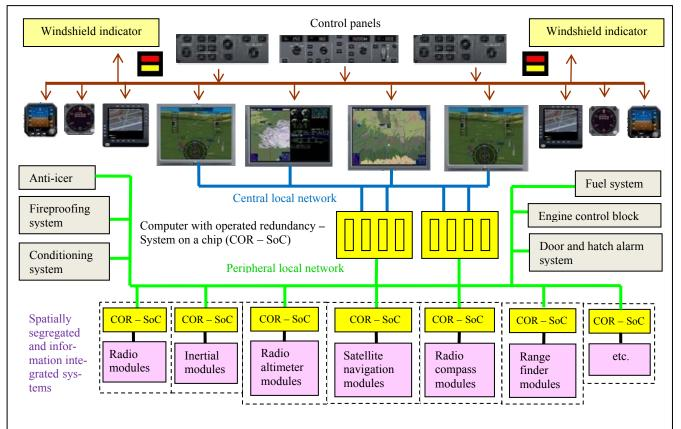
Fig. 1. Assumed Structure of Airborne Complex for the Day After Tomorrow.
