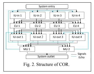
The following abbreviations are used in this figure: IU stands for an Interface Unit, CU stands for a Computing Unit, and MU stands for a Multiplex Unit. Additional letter combinations stand for either entry or outlet parts of Interface Units. Numerals are used to name dubbed or four times reproduced identical units.
