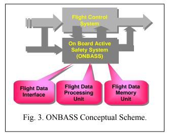
Suggested (designed or planned to be designed) devices provide "activeness" of safety as well as gracefulness of degradation of the system (here an aircraft) when the full recovery is impossible. Diagnostic and test hardware units provide automatic on-board and on-ground supportive reliability tests.
