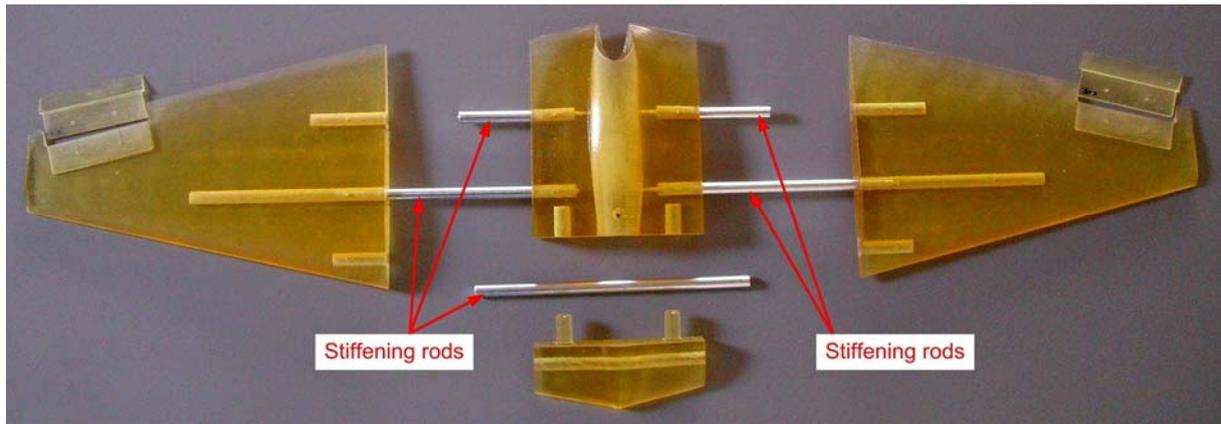
Fig. 8. The ILAS model before final assembly showing the five reinforcing rods
