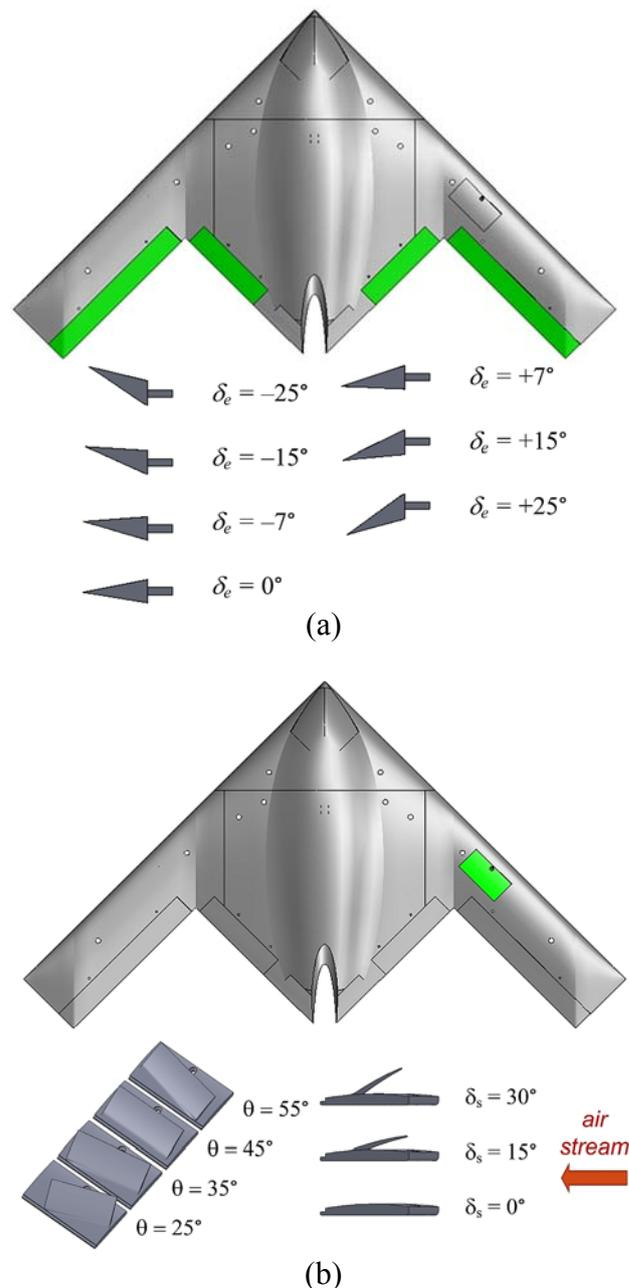
Fig. 2. CERBERUS control surfaces: (a) elevons for pitch and roll control, and (b) spoilers (only one side made for testing) for yaw control
