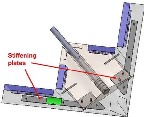
Fig. 9. CERBERUS model showing the two reinforcing steel plates
