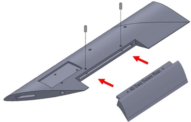
Fig. 11. Detail of an elevator and wing showing the locating features and the fastening by screws. An inscription made as part of the RP process contains the elevator's designation
