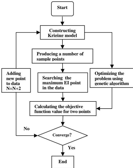
Fig. 6. Framework of the improved Kriging-model-based optimization design algorithm.
