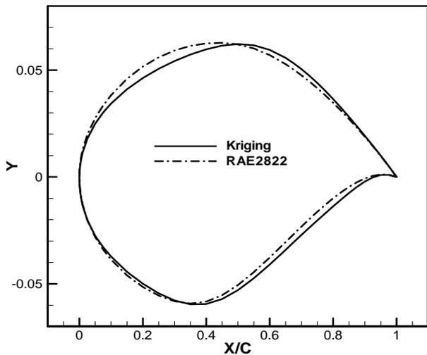
Fig. 9. Comparison of geometry between the optimal and baseline airfoil
