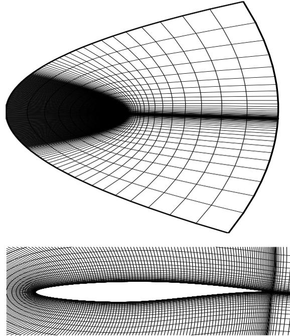
Fig. 7. Schematics of computational grid for RAE2822 airfoil(grid cell: 344×96)
