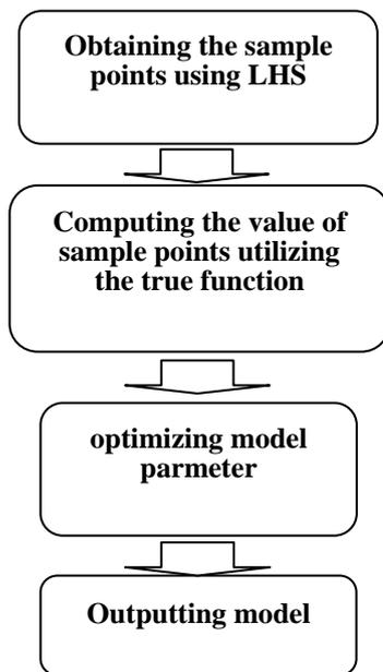
Fig. 2. The flowchart of constructing Kriging model
