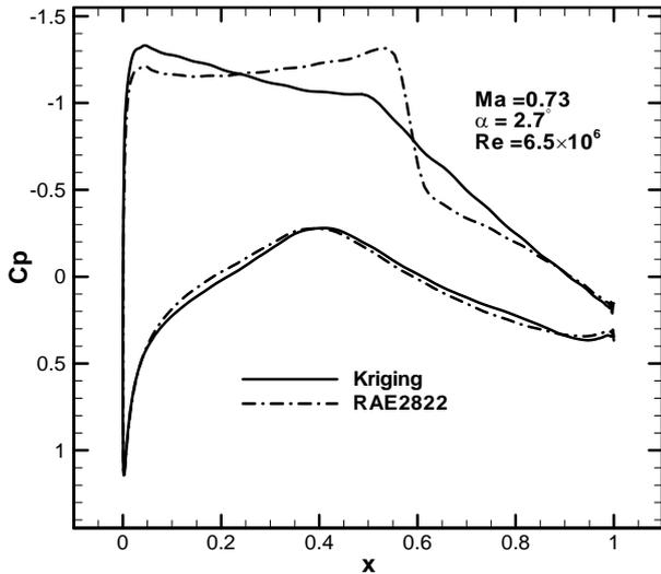
Fig. 8. Comparison of pressure distribution between the optimal and initial airfoil
